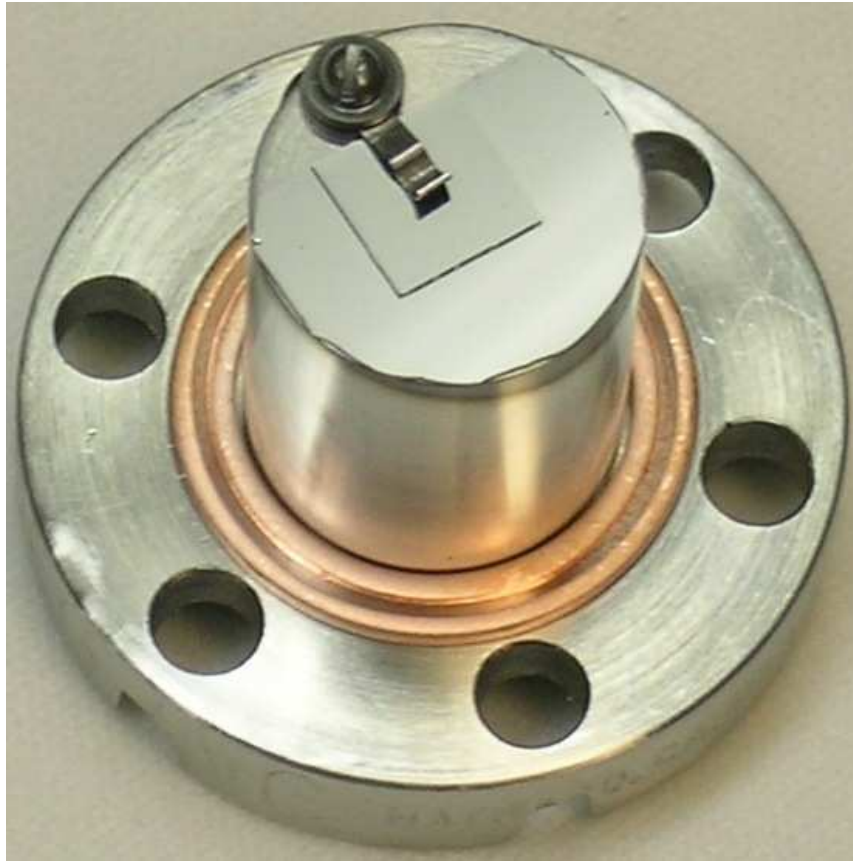
Figure 3. A coupon used to measure the deposition rate of the NEG material.
