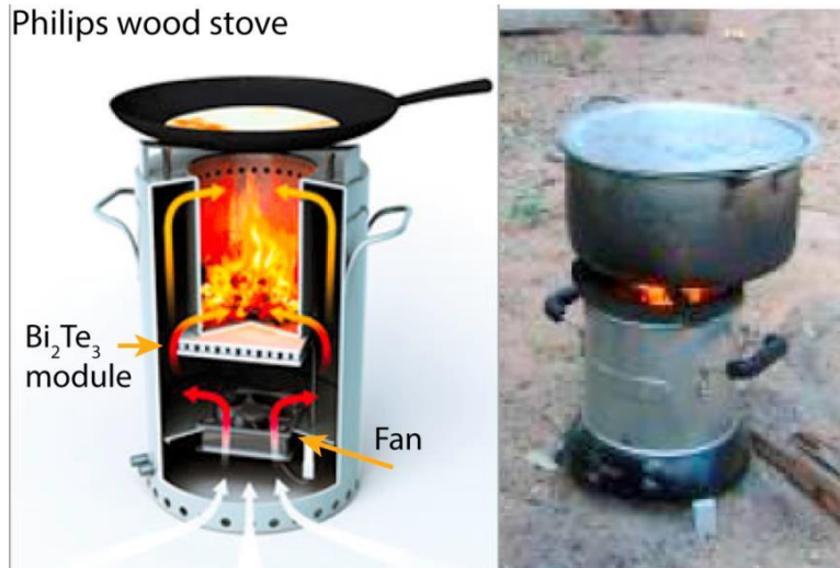
Figure 1.3: An example of a biomass fueled advance stove featuring \text{Bi}_2\text{Te}_3 thermoelectric module, developed by Philip’s Research. Picture taken from reference 18.
