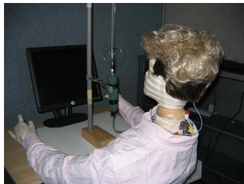
Figure 19, breathing-zone velocity measurement near the heated thermal manikin
