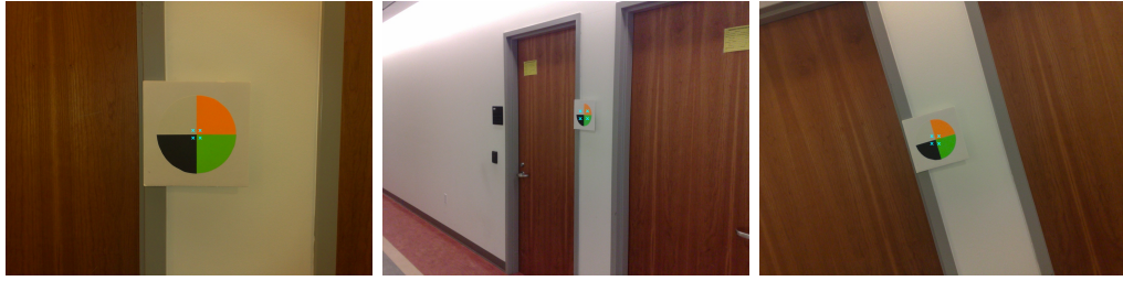
Figure 2.1: Our color marker, seen from different viewpoint and with different camera rotations. The blue superimposed crosses represent a fixed-size ‘probe’.
