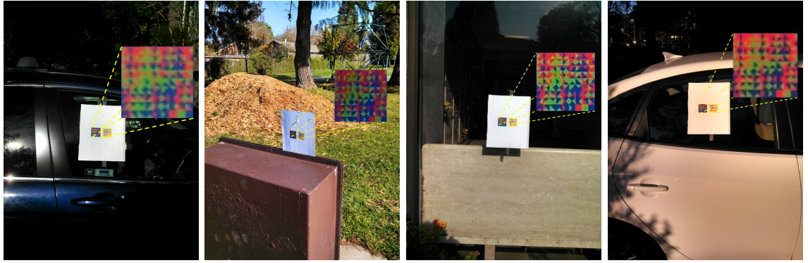
Figure 5.5: Examples of barcode images after perspective projection correction taken at multiple distances and viewing angle.
