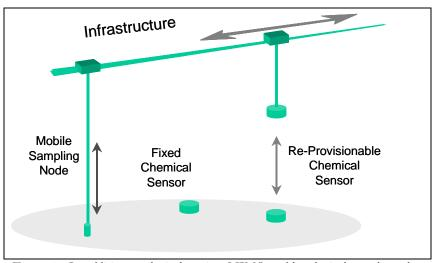
Figure 5. In addition to physical sensing, NIMS enables physical sampling where mobile devices may acquire samples according to an event-driven or scheduled algorithm and convey samples to centralized sample analysis facilities (that may include remote laboratory analysis). NIMS also permits re-provisioning of in situ sensors that may be otherwise limited by a short operating lifetime in the medium.
