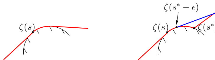
Figure 5.14: Cartoon for the proof of 36. At left, an example of a non-simple (time-optimal) path around an obstacle. At right, we provide a counterexample showing that a tangentially departing path is optimal.
