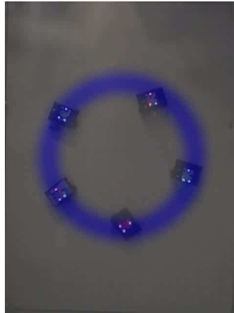
Figure 7.6: Screen capture of the limited-range nonholonomic deployment with the density function overlaid on top.
