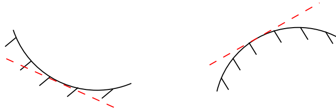
Figure 5.11: Diagram illustrating convexity relative to the flow environment. At left, an example of a locally strictly convex boundary with a dashed tangent line. At right is a locally strictly concave curve with a dashed tangent line.
