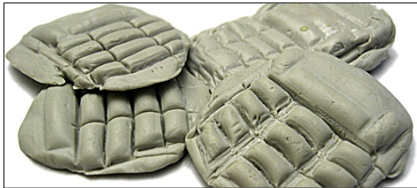
Figure 2.8: The clay prototypes we used to determine minimum button spacing.
