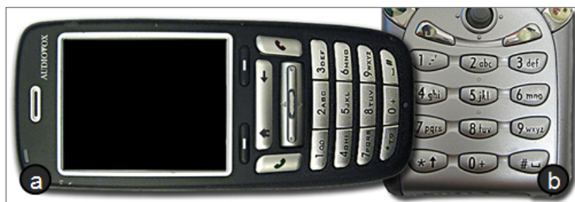
Figure 2.7: (a) The Audiovox 5600 phone. (b) The Red-E SC1100 phone offers more space between buttons.
