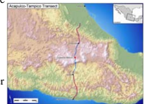
Fig. 2. Line of radio linked (blue) and standard stand alone (red) seismometers spaced every 5 km to study wave-propagation and the subducting slab. This experiment will give the seismic community a strong understanding of the benefits of real-time analysis during temporary deployments.
