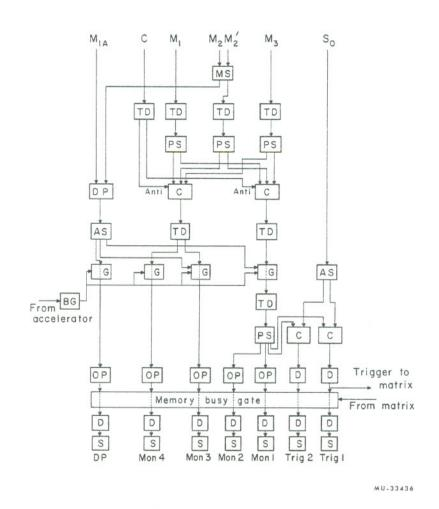
Fig. 6. Block diagram of the monitor electronics system.
