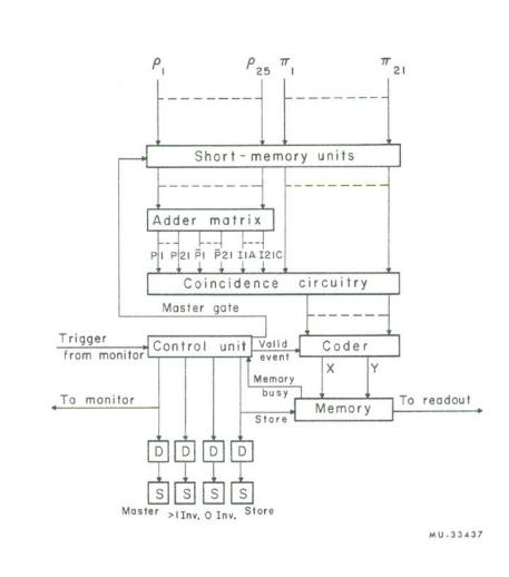
Fig. 7. Block diagram of the coincidence-matrix electronics system.
