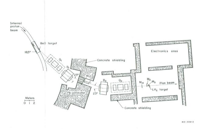
Fig. 2. Plan view of the experimental arrangement. Symbols  $O_1$ ,  $B_1$ ,  $B_2$ , and  $O_2$  represent magnets. The beam counters are labelled  $M_1$ ,  $M_{1A}$ ,  $M_2$ ,  $M_3$ , and C. The counters, BeO target, and LH<sub>2</sub> target are not drawn to scale.
