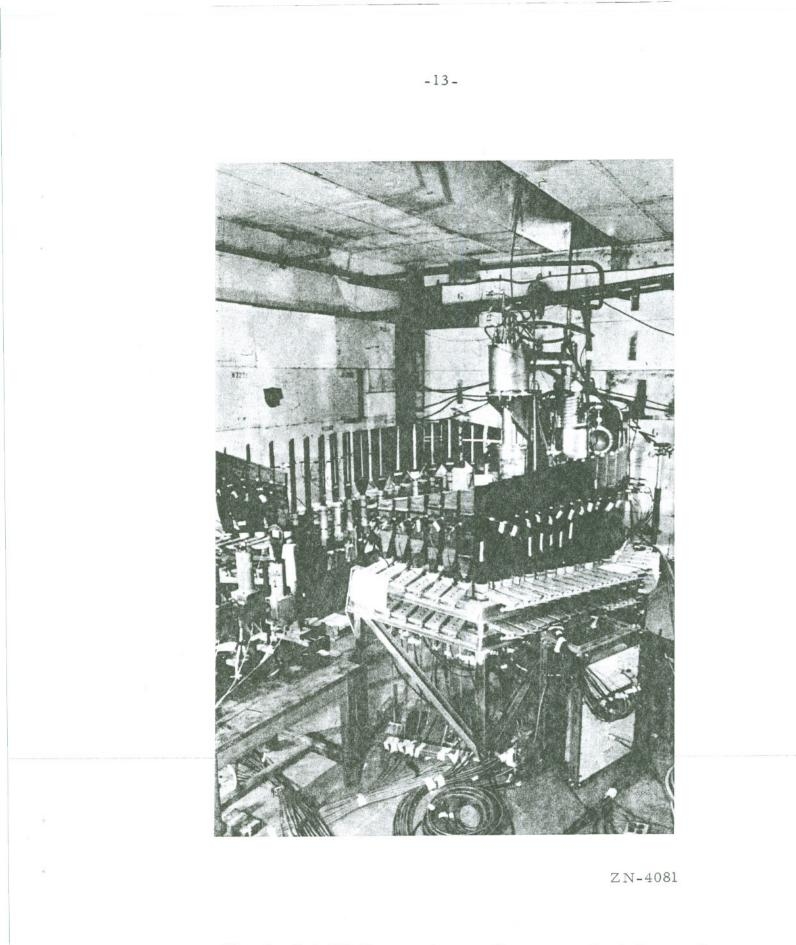
Fig. 5. Scintillation counters as they were situated around the hydrogen target.
