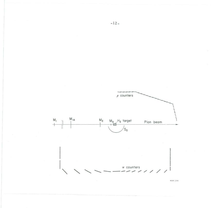
Fig. 4. Plan view of scintillation-counter array.
