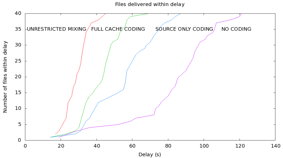
Figure 6.7: Simulation results: corridor model with 30% loss probability
