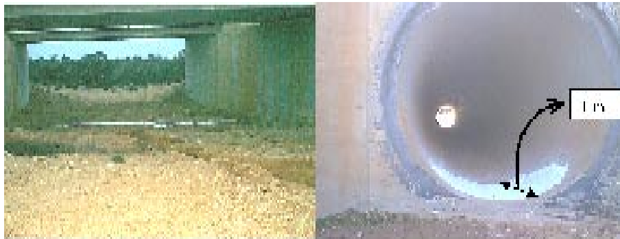
Fig. 1. Marble dust beds used for footprint monitoring in a wildlife underpass and a circular culvert. In both cases dust beds are 1m wide.
