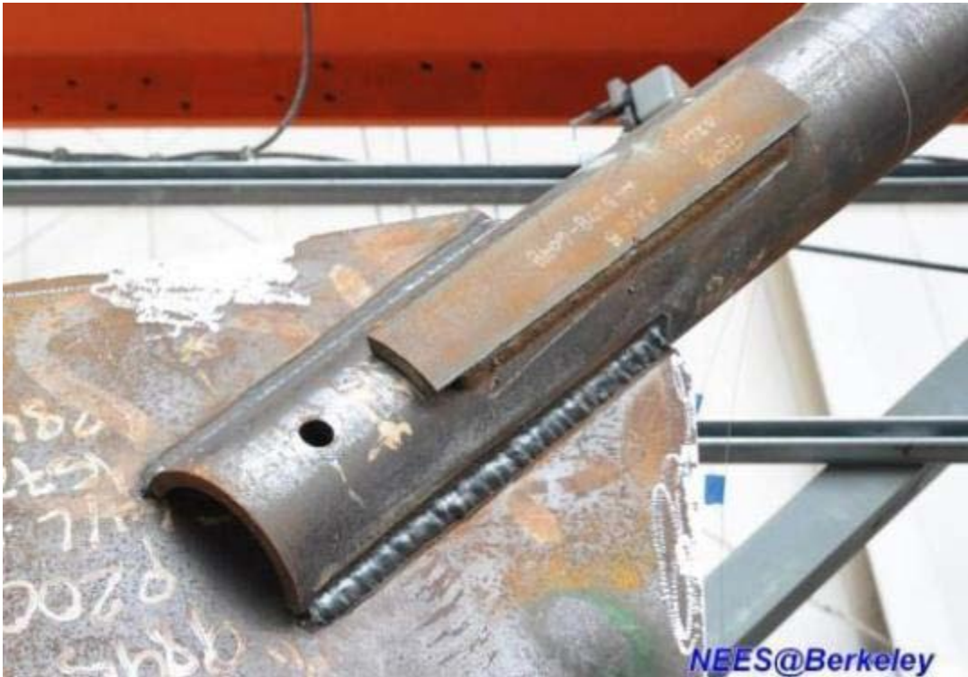
Figure 3.27 Detail view of reinforcing plate of TCBF-B-2 specimen
