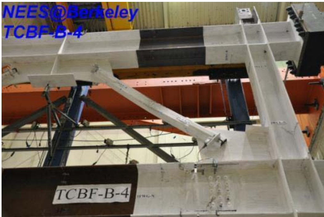
Figure 4.413 Global buckling of western side brace in the second story
