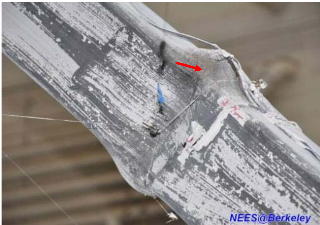
Figure 4.95 The square HSS brace in the first story at western side of TCBF-B-1 specimen
