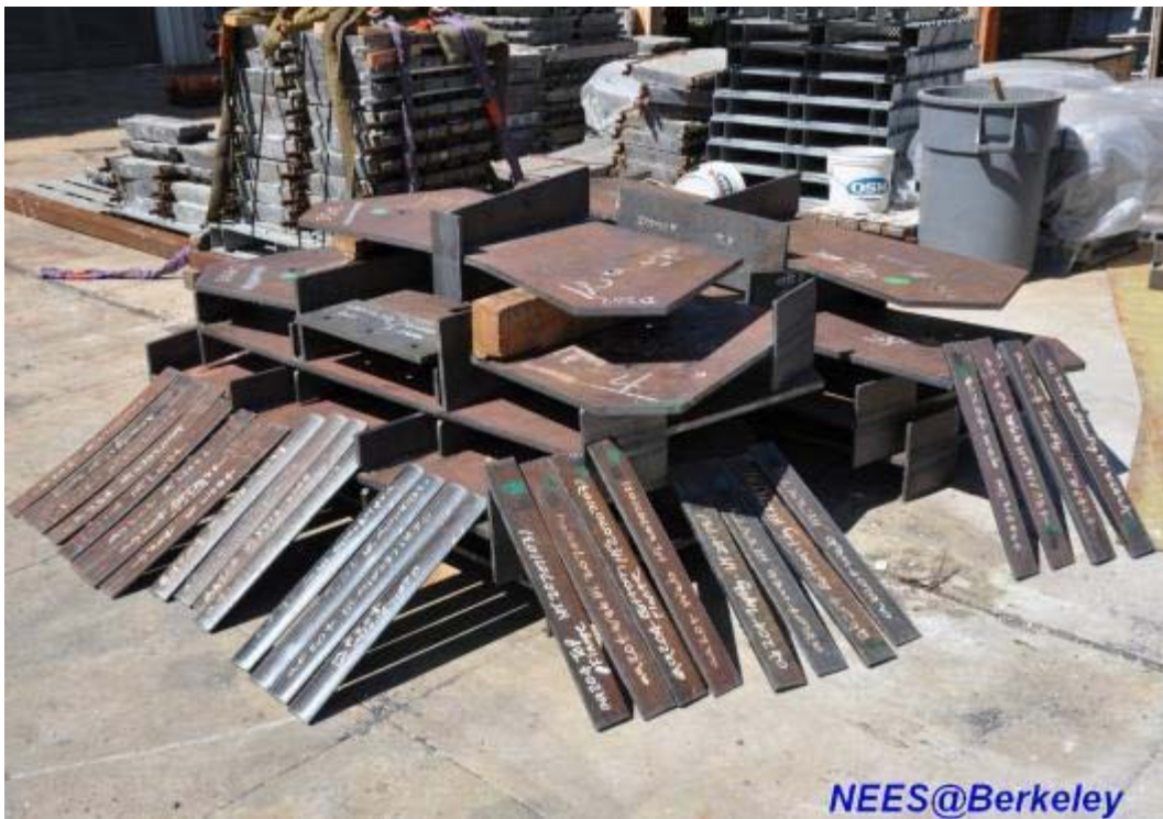
Figure 4.4 Steel coupons of TCBF-B-2, TCBF-B-3 and TCBF-B-4 specimens
