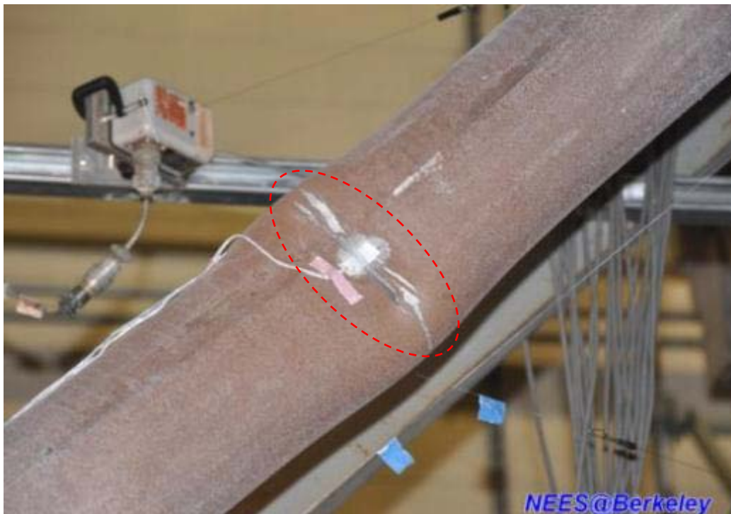
Figure 4.218 Partial fracture of the west side brace in the first story (Specimen TCBF-B-2)
