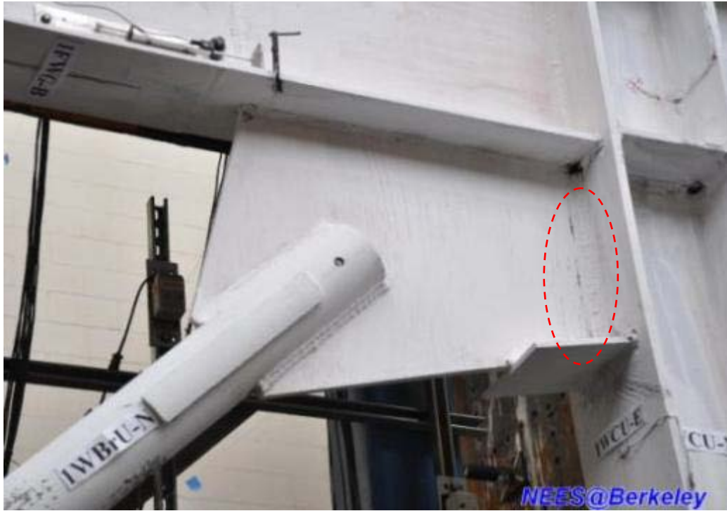
Figure 4.195 Flaking of whitewash near gusset plate-to-column flange region (Specimen TCBF-B-2)
