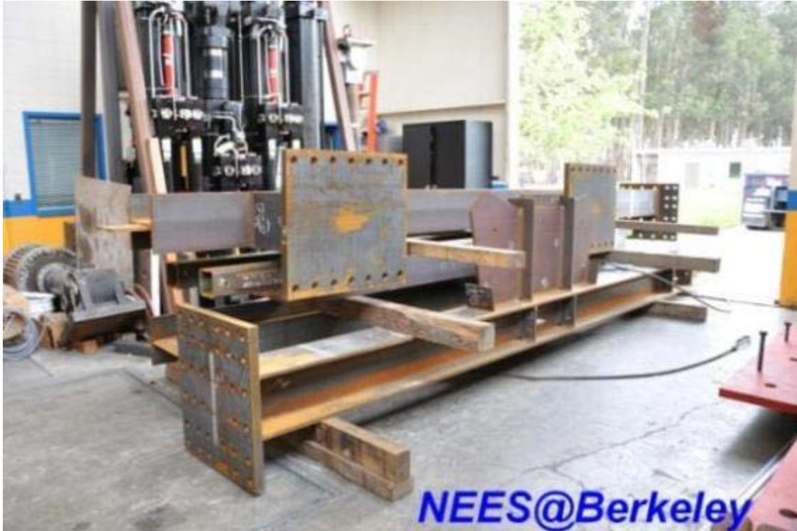
Figure 3.25 (a) The sub-assemblages of specimens TCBF-B-1 and TCBF-B-2
