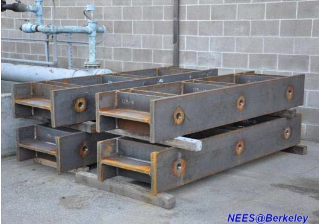
Figure 3.13 Load transfer beams below strong floor before erection
