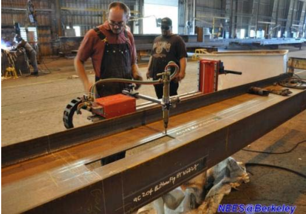
Figure 4.1 Torch cutting the steel coupon from wide flange section
