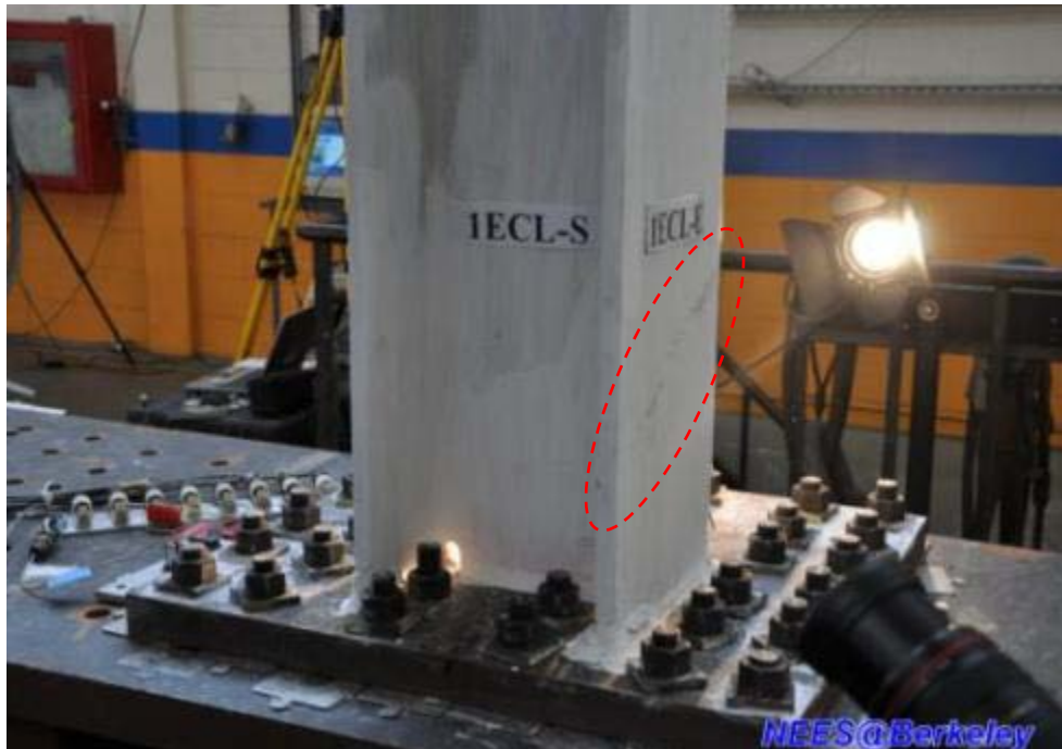
Figure 4.191 Yield pattern of the east column flange (Specimen TCBF-B-2)
