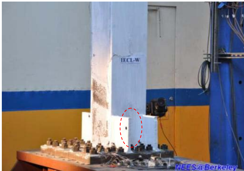
Figure 4.206 Yield pattern between column base stiffener plates (Specimen TCBF-B-2)
