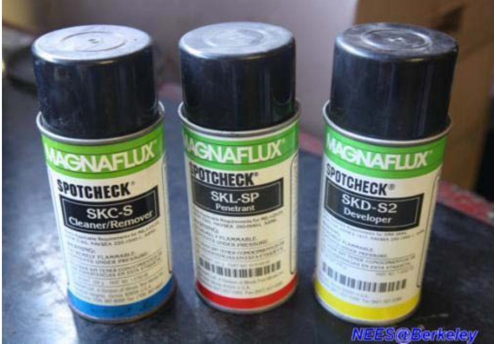
Figure 3.49 Three-step crack detecting spray
