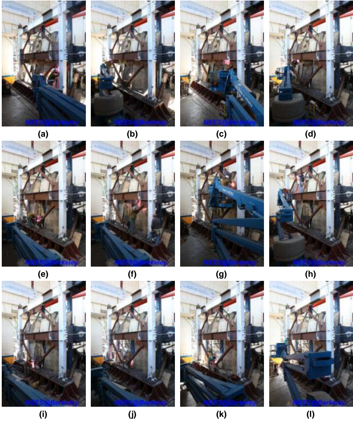
Figure 3.66 Key welding processes of TCBF-B-4 specimen
