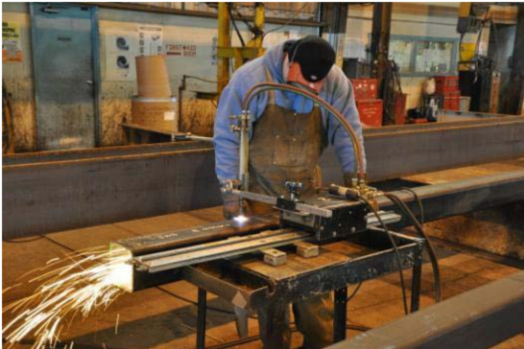
Figure 4.2 Torch cutting the steel coupon from HSS section
