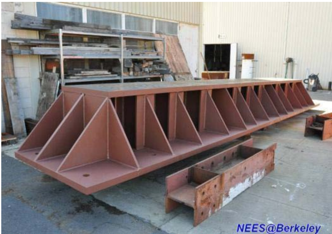
Figure 3.12 The built-up floor beam after painting
