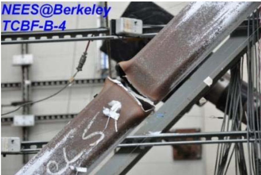
Figure 4.427 Completely fracture of the first story western side brace
