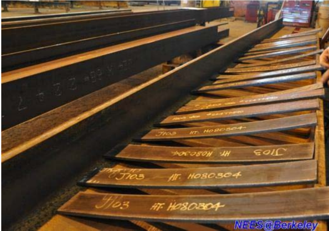
Figure 4.3 Steel coupons of TCBF-B-1 specimens
