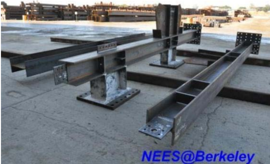
Figure 3.25 (b) The sub-assemblages of specimens TCBF-B-3 and TCBF-B-4
