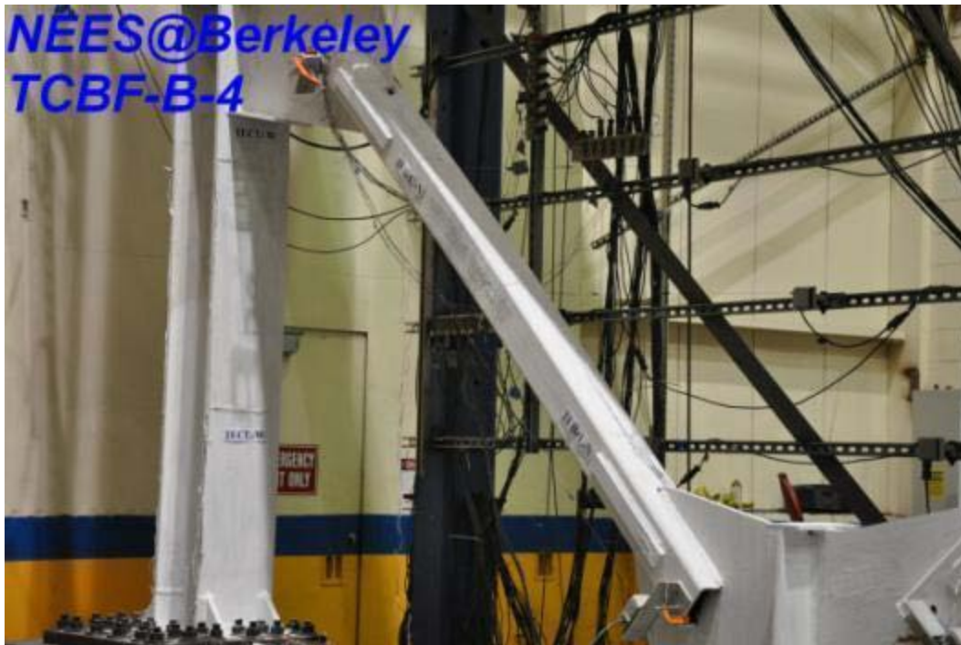
Figure 4.412 Global buckling of eastern side brace in the first story
