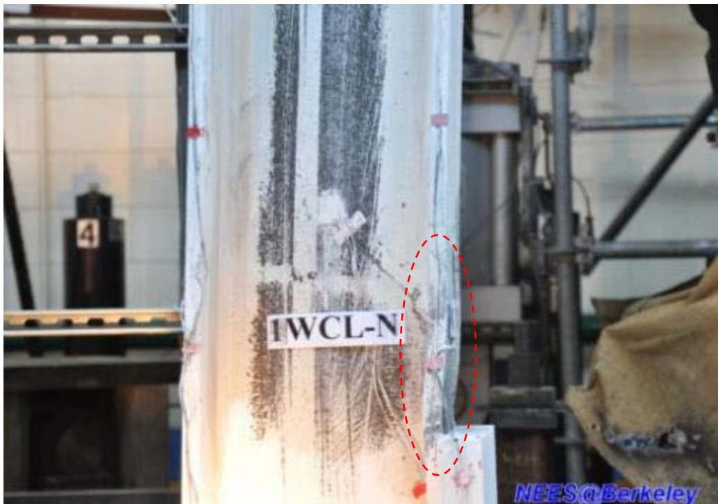
Figure 4.210 Local buckling of column flange near 2-in.-thick cover plate (Specimen TCBF-B-2)
