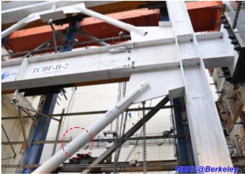
Figure 4.189 Whitewash flaking at the middle of the west side round HSS brace (Specimen TCBF-B-2)
