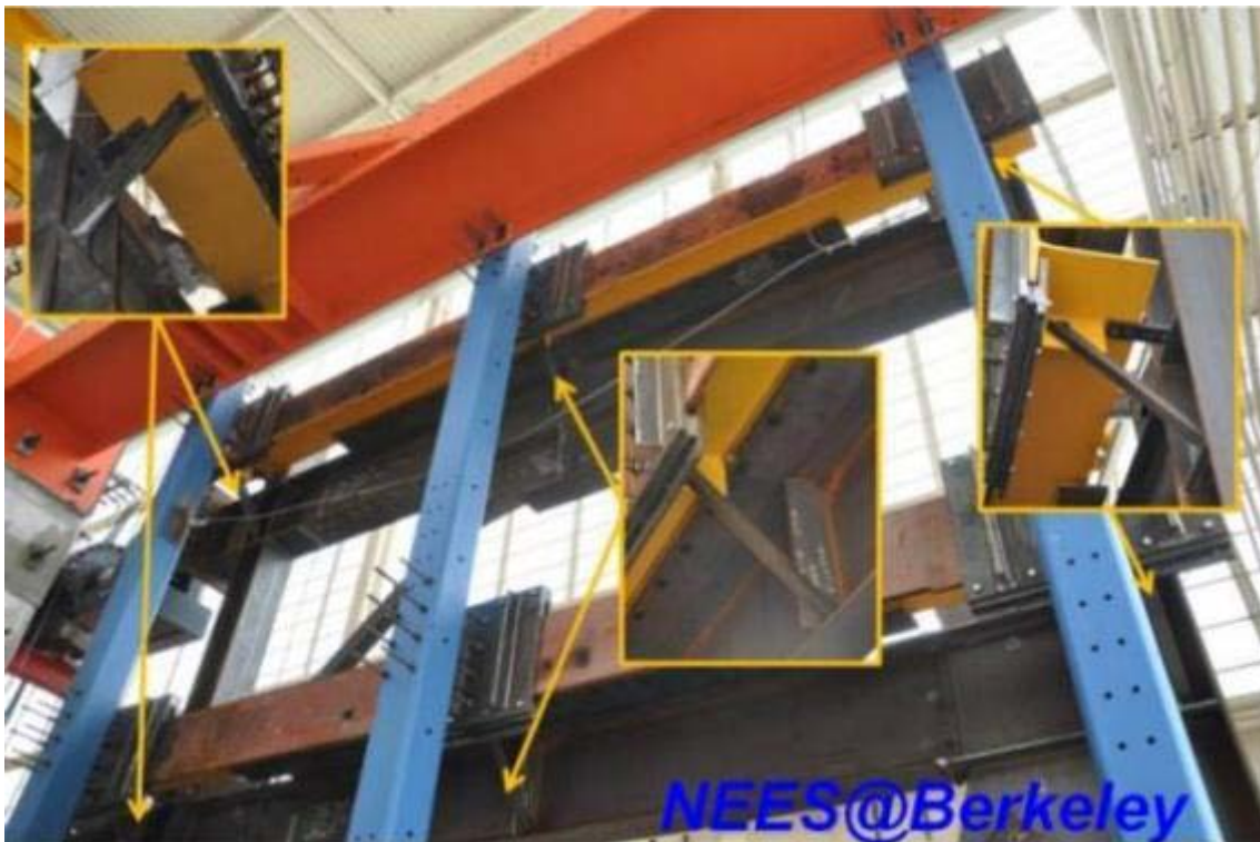
Figure 3.38 Steel angle kickers below the tee section
