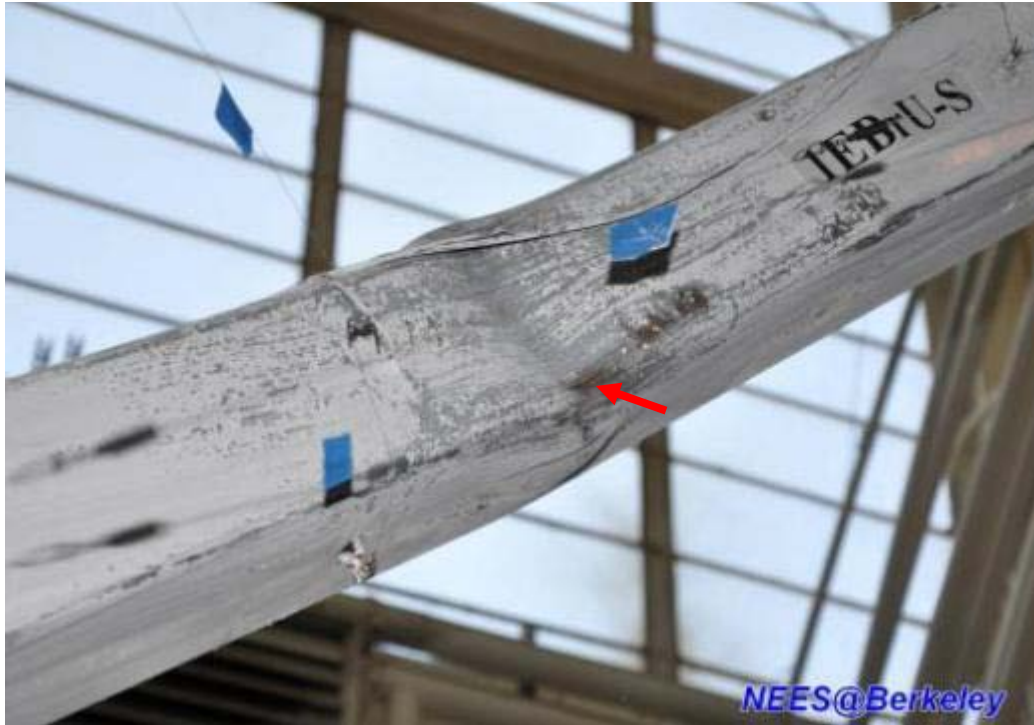
Figure 4.94 The square HSS brace in the first story at eastern side of TCBF-B-1 specimen
