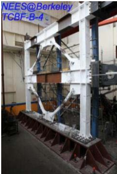
(c) After design earthquake (DE)
