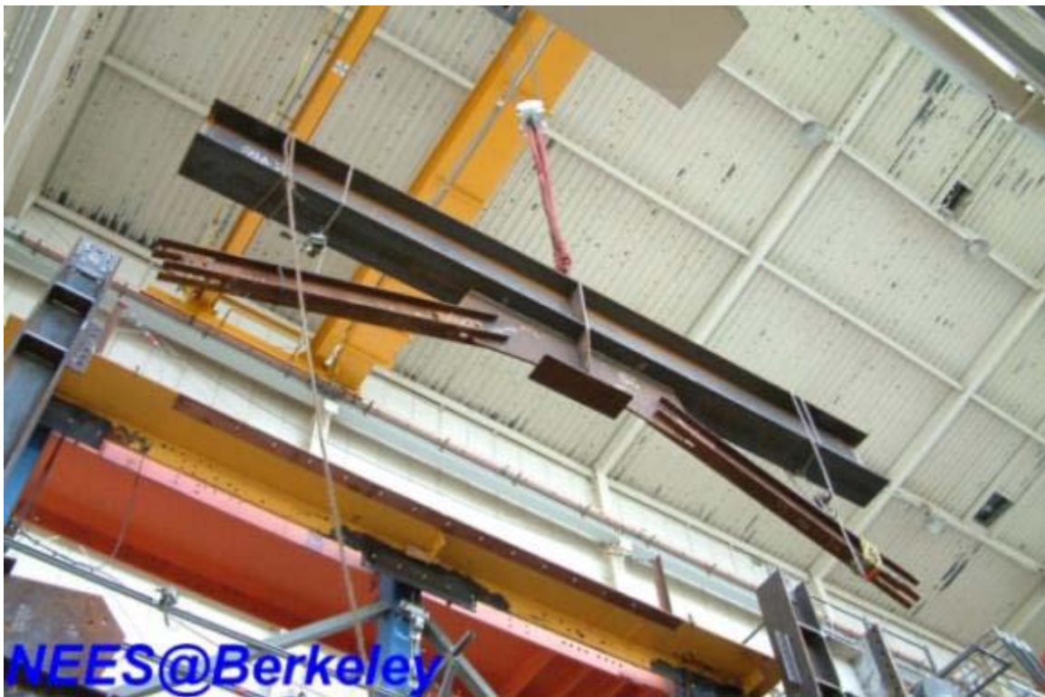
Figure 3.56 Roof beam, gusset plate and brace sub-assembly of TCBF-B-3 specimen
