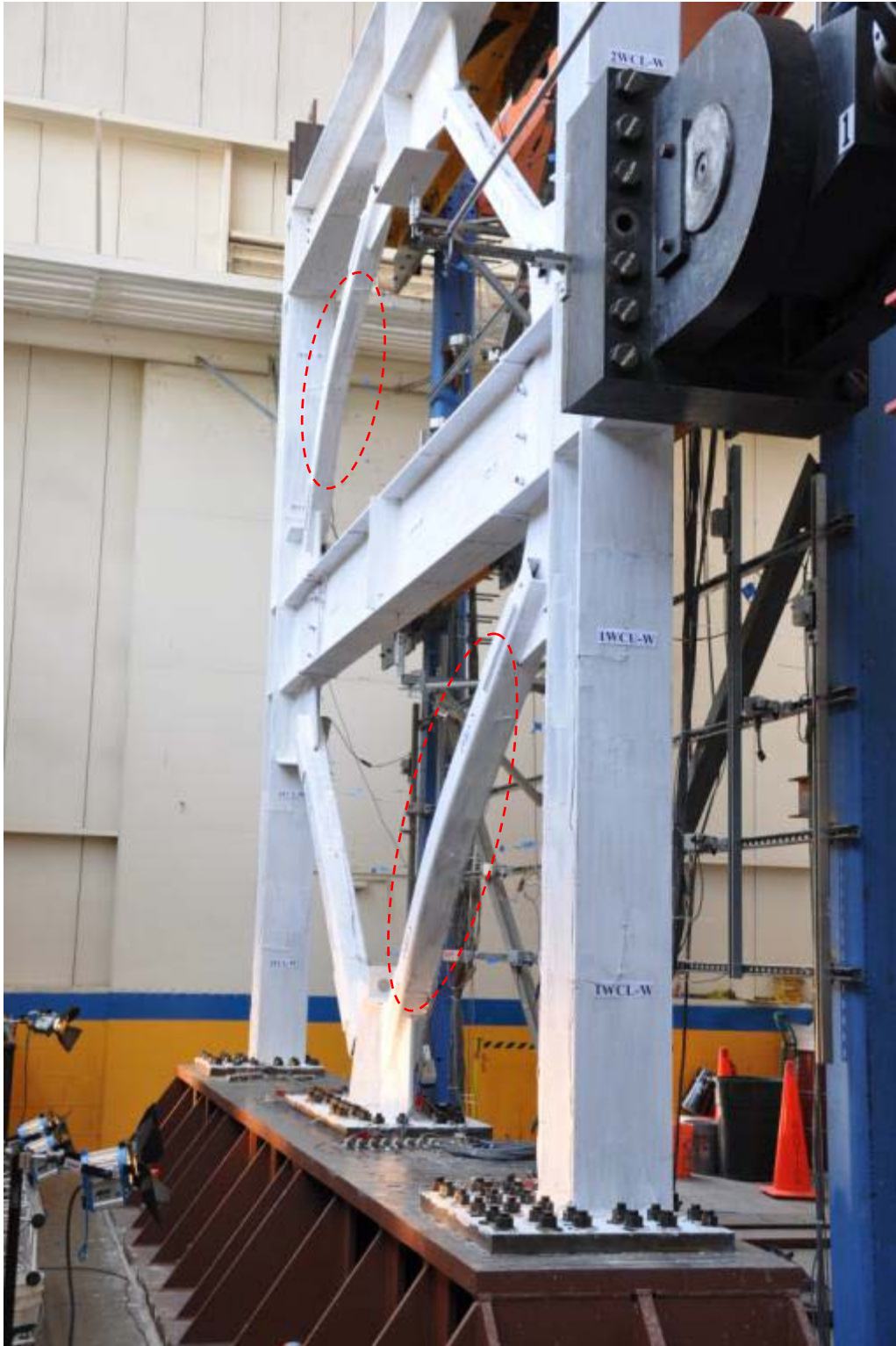
Figure 4.87(b) The flaking of whitewash at the middle length of braces of TCBF-B-1 specimen
