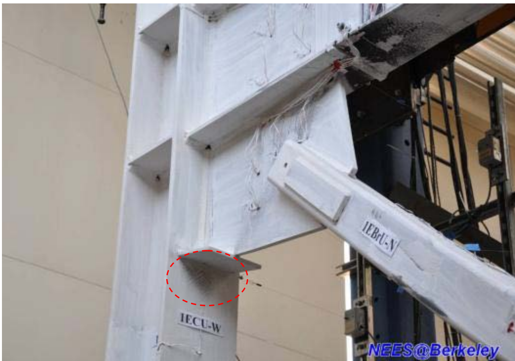
Figure 4.93 The gusset plate-to-column connection at eastern side of TCBF-B-1 specimen
