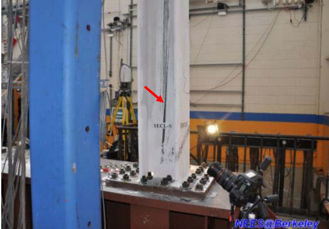
Figure 4.199 Column web yielding at the east side column in ground floor (Specimen TCBF-B-2)
