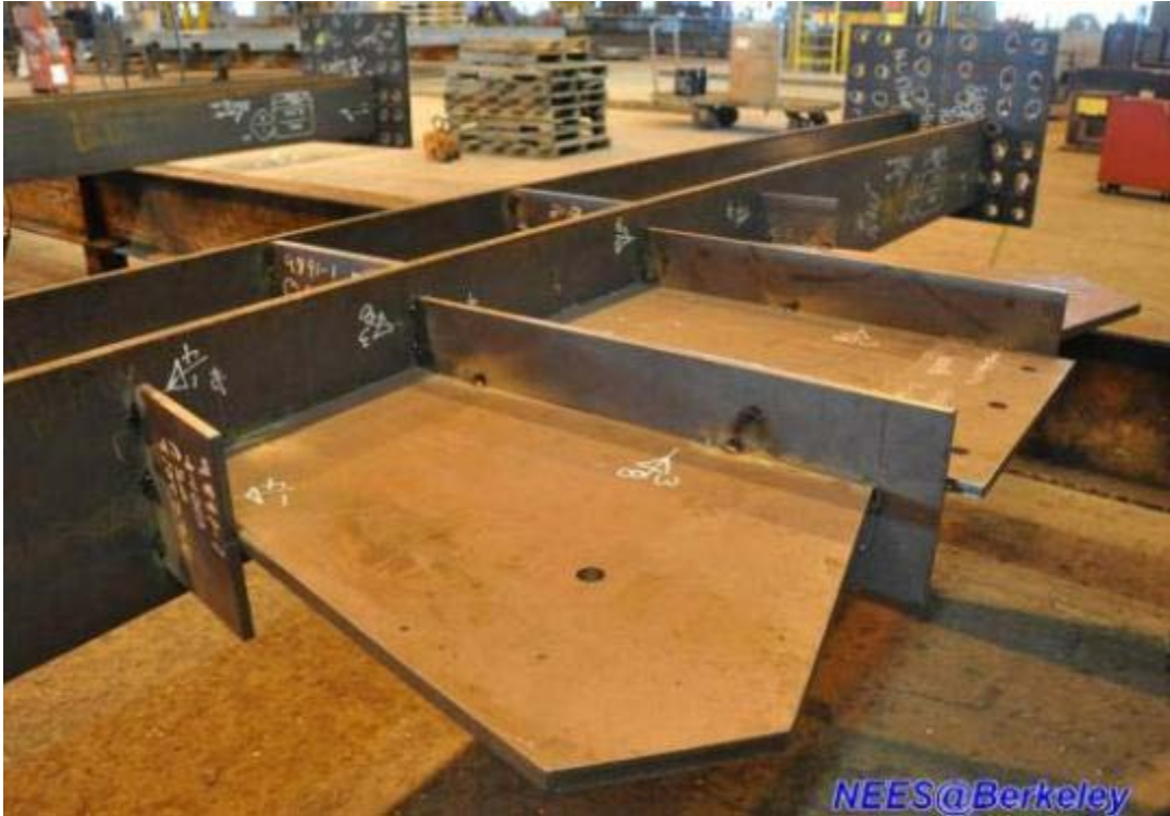
Figure 3.26 The \frac{3}{4} inch one-piece gusset plate after tack welding to column flange
