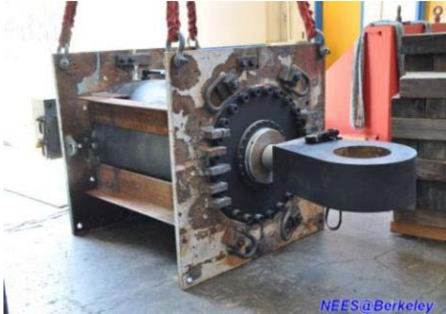
Figure 3.31 Steel jacket for rotating the 1.5 M-lb actuator during the load cell calibration
