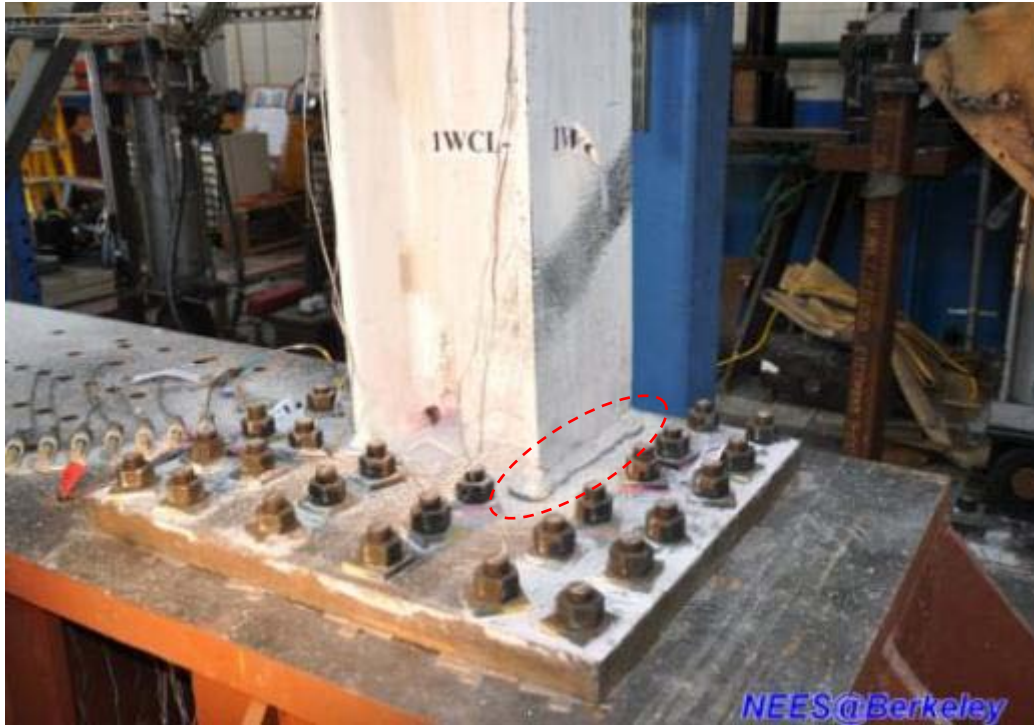
Figure 4.201 Complete fracture near the flange CJP welds at west side column base (Specimen TCBF-B-2)
