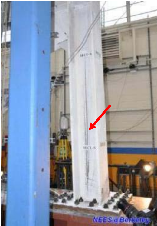
Figure 4.97 The flaking of whitewash on column web at eastern side of TCBF-B-1 specimen
