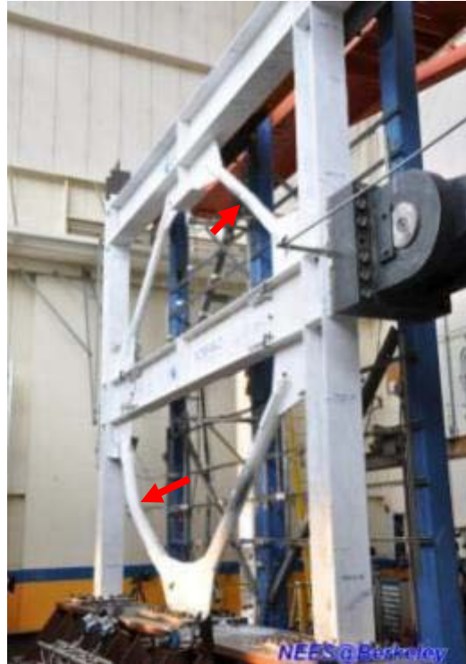
Figure 4.193 Global buckling of round HSS braces at both stories of TCBF-B-2 Specimen
