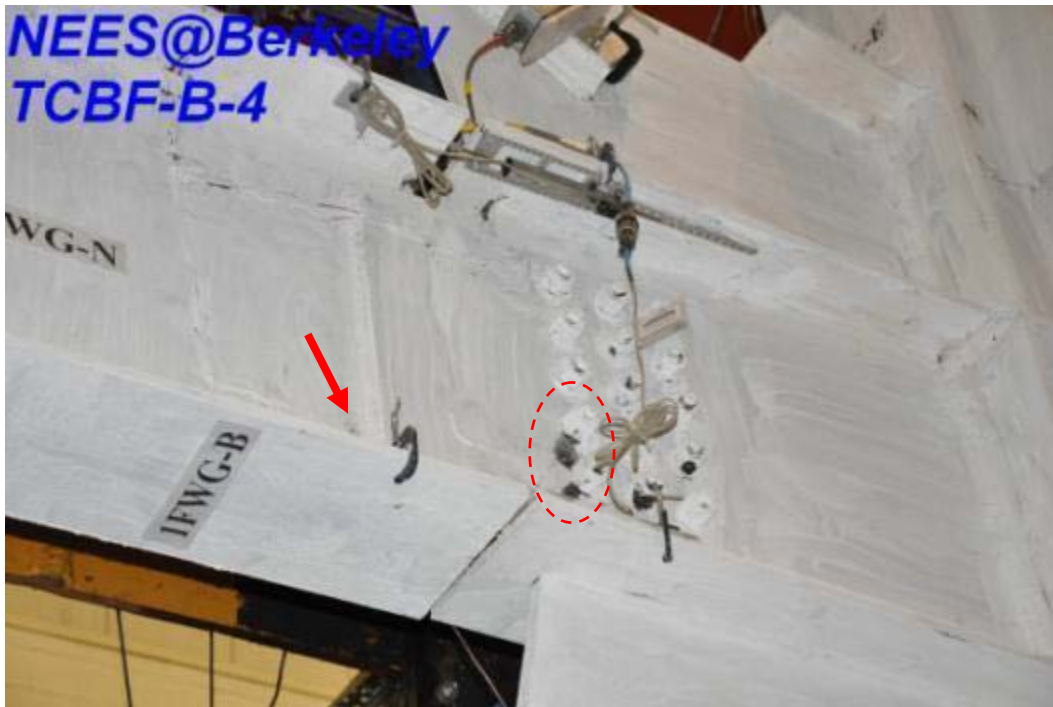
Figure 4.416 Local yielding in the beam-to-gusset plate splice
