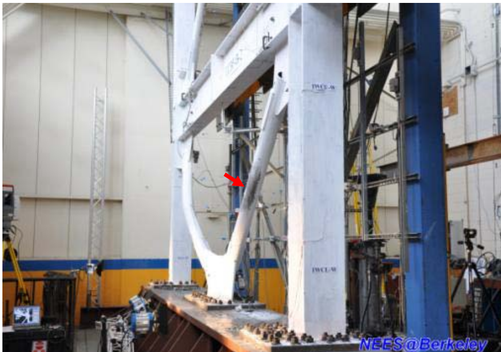
Figure 4.194 Additional whitewash flaking in the braces (Specimen TCBF-B-2)
