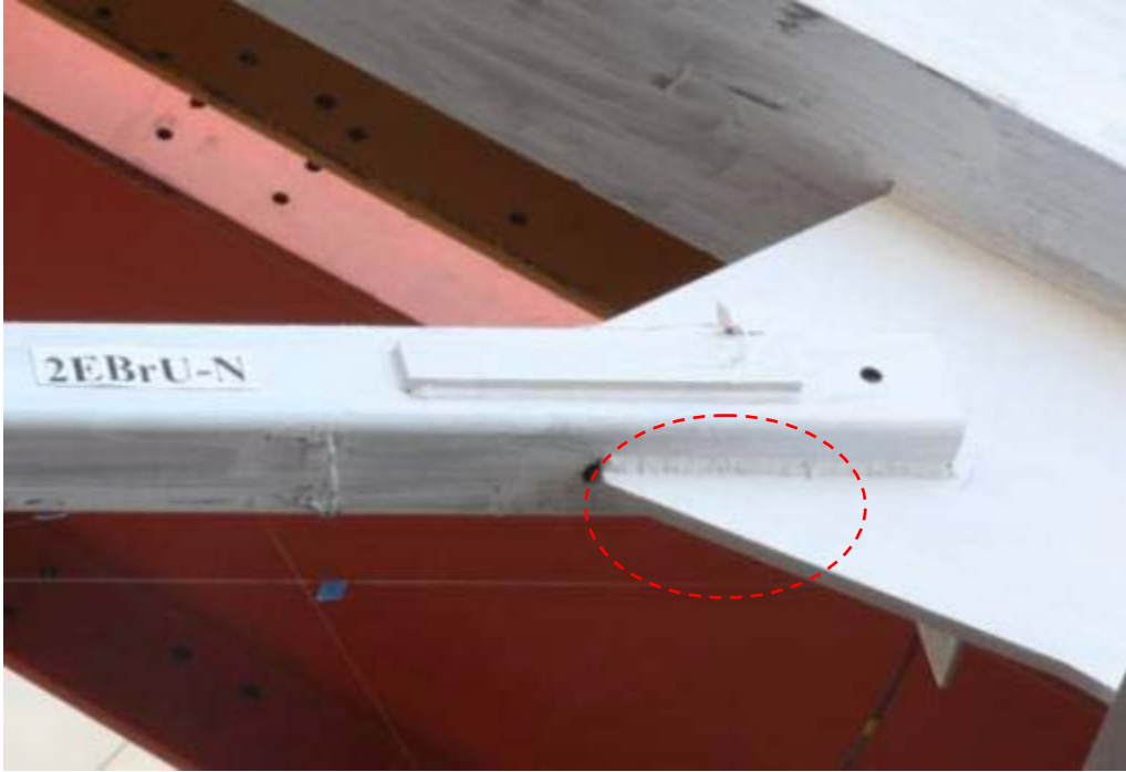
Figure 4.87(a) The flaking of whitewash at second story gusset plate of TCBF-B-1 specimen
