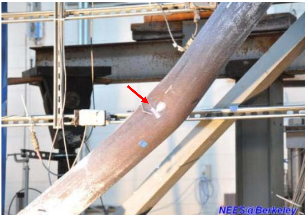
Figure 4.212 Local buckling of west side round HSS brace in the first story (Specimen TCBF-B-2)
