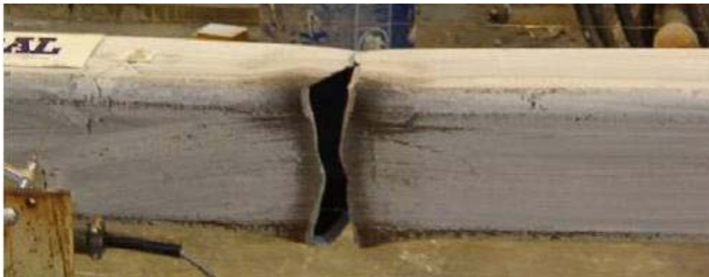
(b) Test photo at middle length of HSS brace (extracted from Fig. 12 in Yang and Mahin, 2005)
