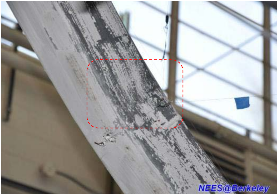
Figure 4.91 The middle portion of a HSS brace at western side of TCBF-B-1 specimen in first story
