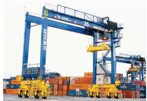
Figure 1.1: (a) A gasoline/electric hybrid bus (taken from Ref. [1]) and (b) hybrid diesel/electric rubber-tired gantry crane (taken from Ref. [2]) equipped with electrochemical capacitor energy storage systems.
