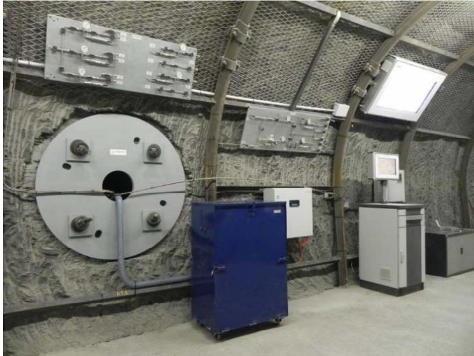
Figure 3-3. SEALEX Experiment at the Tournemire URL: View of mini-tunnel from gallery after core emplacement (from Barnichon, 2011)
