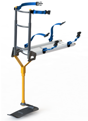
FIGURE 10. The passive walking device, incorporating two four bar linkages on both sides of the knee. The four bar linkage at the knee follow a scaled down "tear-drop trajectory", obtained from actual human walking trajectory at foot level.
