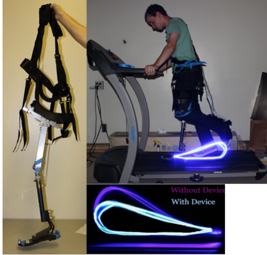
FIGURE 4. Prototype of the second passive walking device developed to assist a person with lower leg injury.
