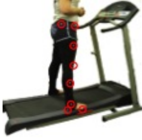
FIGURE 6. Experimental set up: Subject walking on a treadmill, monitored by a 3D Motion Capture System. Reflective markers were attached on the subject's right leg.
