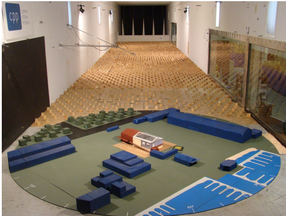
Figure 5.28: Alameda Test Building in Wind Tunnel – December 2011
