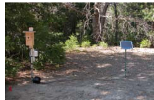
Nestbox with Cyclops, environmental monitoring sensors, and solar panel.
