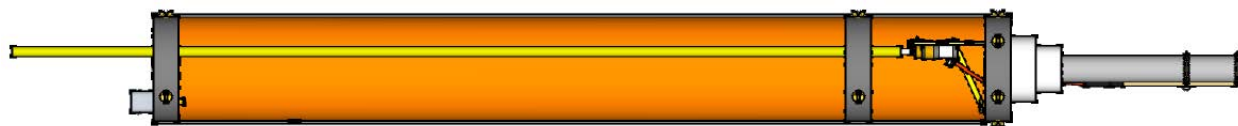
Figure 3.7: Side view of the inside of the probe body (bottom-to-top from left-to-right). The bottom disc supports the BNC coupler, the middle disc guides the tuning rods, and the top disc holds both the circuit board and the combustion tube holder. Gas lines and coaxial cables are not shown for clarity. Also not shown: tuning rod holder (Figure 3.9) and shield (Section 3.1.8).
