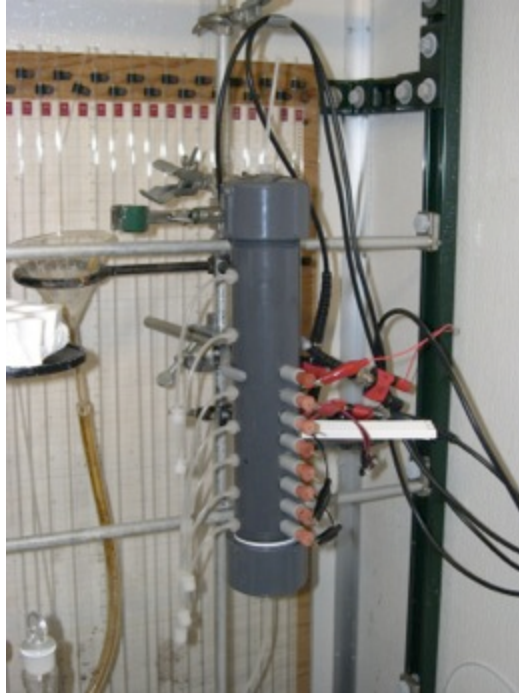
Figure 15. Column with electrodes for induced polarization measurements.
