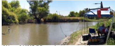
[Above] NIMS RD moving sensor package across river transect.
