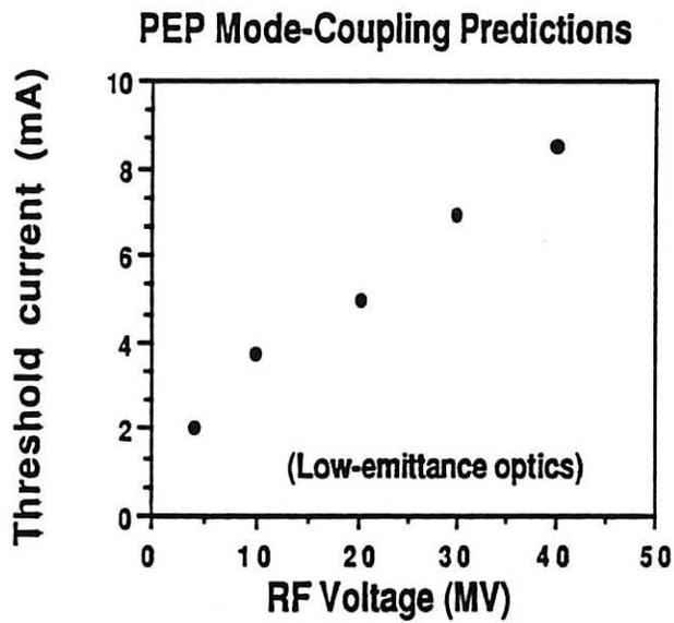
Fig. 6 Predicted mode-coupling threshold current as a function of applied RF voltage. Calculations from Ref. 5.
