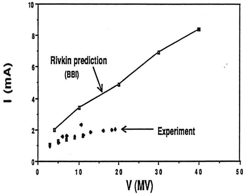
Fig. 8 Predicted and observed single-bunch thresholds for the PEP low-emittance optics at 7.1 GeV. Predicted values are taken from Ref. 5.
