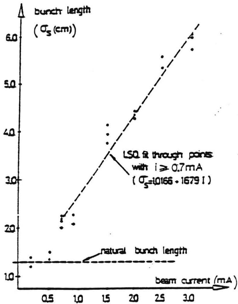
Fig. 1 Results of PEP bunch lengthening measurements, using collider optics, at 4.5 GeV. Taken from Ref. 6.
