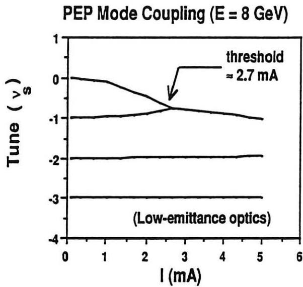
Fig. 5 Mode-coupling predictions for the PEP low-emittance optics at 8 GeV.
