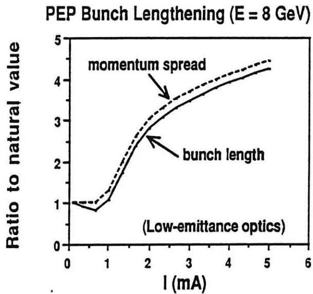
Fig. 4 Bunch lengthening predictions from BBI, for the PEP low-emittance optics at 8 GeV. Results are plotted as the ratio of  $\sigma_L/\sigma_{L0}$  (bunch length) and  $\delta p/\delta p_0$  (momentum spread), where  $\delta p = \sigma_p/p$ .
