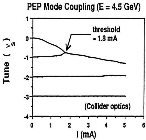
Fig. 3 Mode-coupling calculations for PEP collider optics. The  $Q=1$  broadband resonator was centered at 1 GHz, and had a transverse impedance of  $0.6 \text{ M}\Omega/\text{m}$ . Calculations from Ref. 5.
