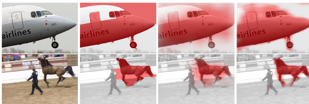
Figure 3.4: Comparing the hypercolumn representation to the topmost layer of the CNN. Each row shows the image, the original proposal ranked high by the classifier, the predicted figure-ground predicted using the topmost layer ( fc7 ) and the predicted figure-ground predicted using the hypercolumn representation. The hypercolumn-based prediction is sharper and captures thin structures such as legs, even in fairly novel poses. The results shown are before superpixel projection.
