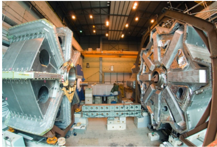
Figure 8.19: Both of the End-cap toroids. The magnet on the left is exposed and has not been installed in its cryostat, while the one on the right is partially installed.
