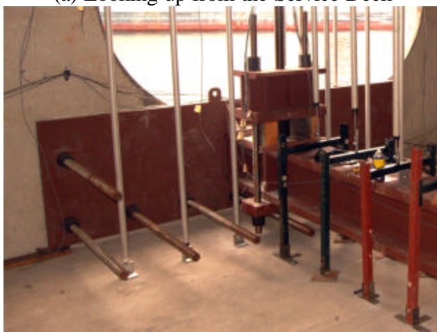
(b) Reaction Plate and Beam - Service Deck
