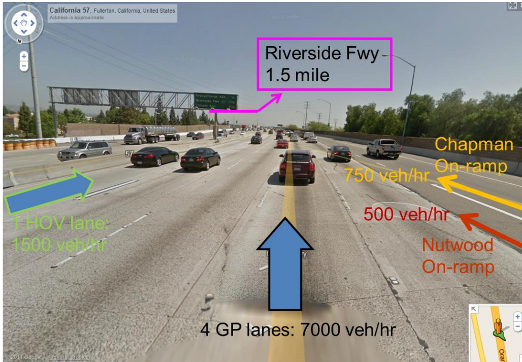
Figure 65. Geometry, Sign, and Traffic Flows around Postmile 6.531 of the SR-57 SB1 Site
