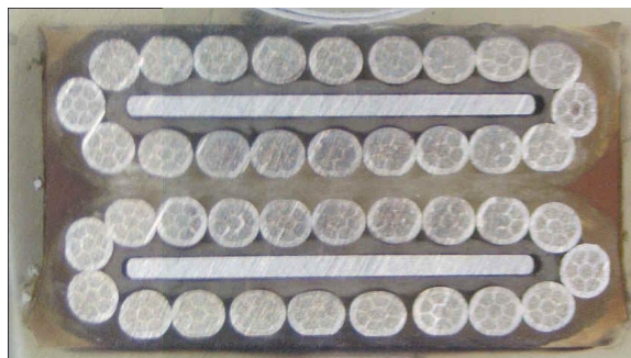
Fig. 1. Optical photograph of two cables of 689. The cross-section shows the potted cables as measure in face loading. The cable thickness and width were 2.35 mm and 8.94 mm, respectively.
