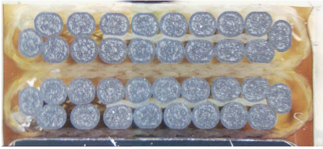
Fig. 2. Optical photograph of two cables of 734. The cross-section shows the potted cables as measure in face loading. The cable thickness and width were 1.47 mm and 8.13 mm, respectively.
