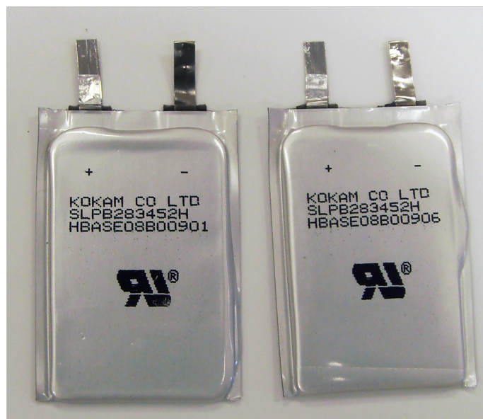
Figure 5.10: The Li-ion polymer battery after uni-axial pressure test.
