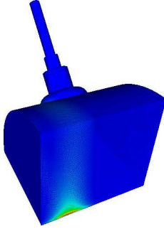
Figure 2: Section of the BPM model used for the wake-potential calculations.
