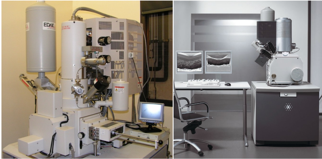
Figure 2.11 Pictures of a Hitachi S4700 Scanning Electron Microscope (left) and FEI Nova 600 SEM/FIB (right).
