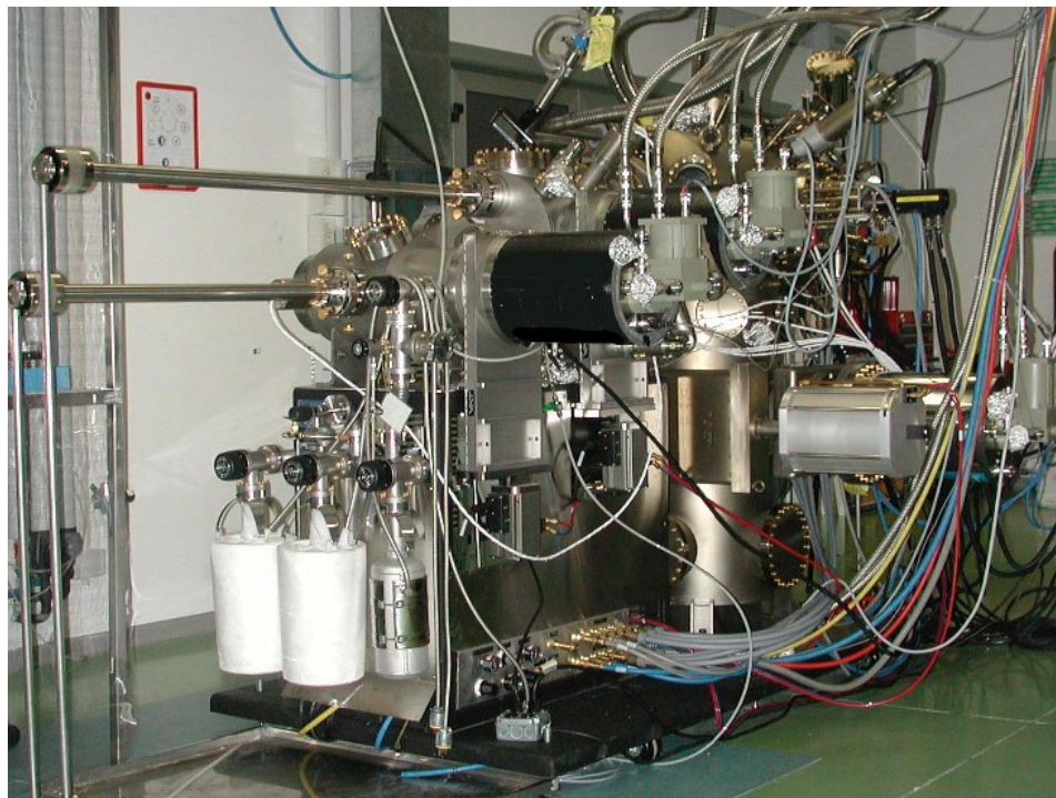
Figure 2.2 Top: A schematic drawing of a generic MBE system, Bottom: Veeco GEN II MBE, installed at the Northrop Grumman Space Technology, Redondo Beach, CA.
