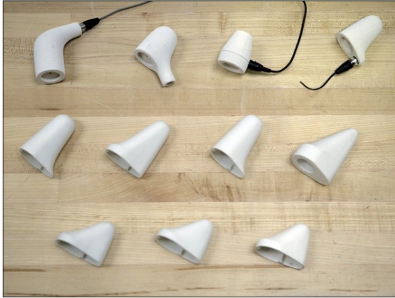
Figure 6.3. IDEO.org’s operational models test ergonomics (Reineck, 2012)
