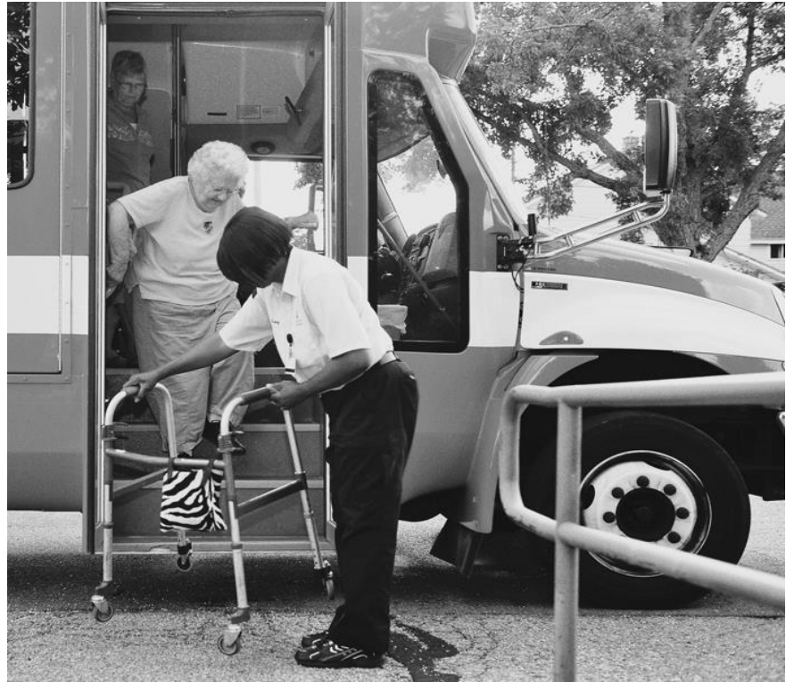
Figure 10: Standard shuttle bus with pedestrian steps not catering to the older adult.
