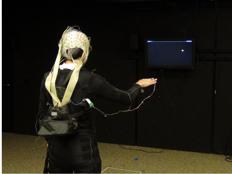
Figure 2.2: A participant wears the full-body motion capture suit with an additional sensor worn on the conducting hand, and a 128-channel EEG system with cables connected to an amplifier worn in a backpack. The participant's movements are animated as a white dot on the facing screen.
