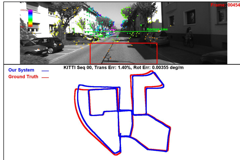
Figure 1.2: Input and output of our visual odometry system. (Top) Input images from video cameras. The colored points are estimated 3D points from our visual odometry system. (Bottom) Vehicle motion estimated from our visual odometry system comparing with ground truth.
