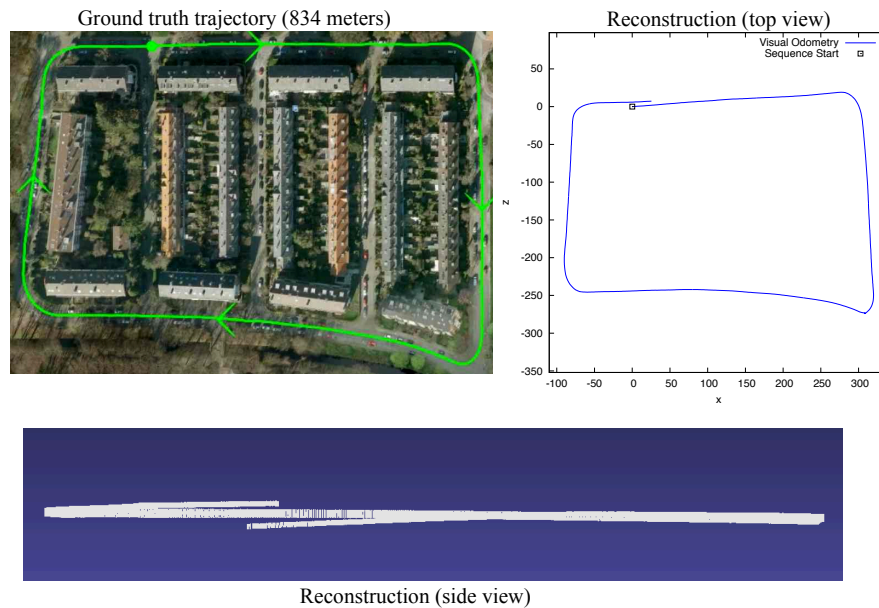
Figure 6.8: The reconstructed trajectories for Seq 2 in Hague dataset, along with ground truth overlays on an aerial map
