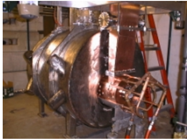
Figure 2. 6-cell open-cell structure installed in the superconducting magnet at the Lab G facility.
