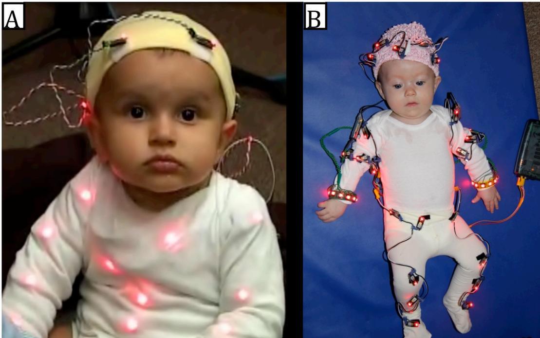
**Figure 7.2:** Versions of the infant suit. A) An early suit prototype, note the diffusion of light from the LEDs on the infant's arms and body created by the external onesie. B) The current suit design, note the absence of the external onesie, and the additional markers
