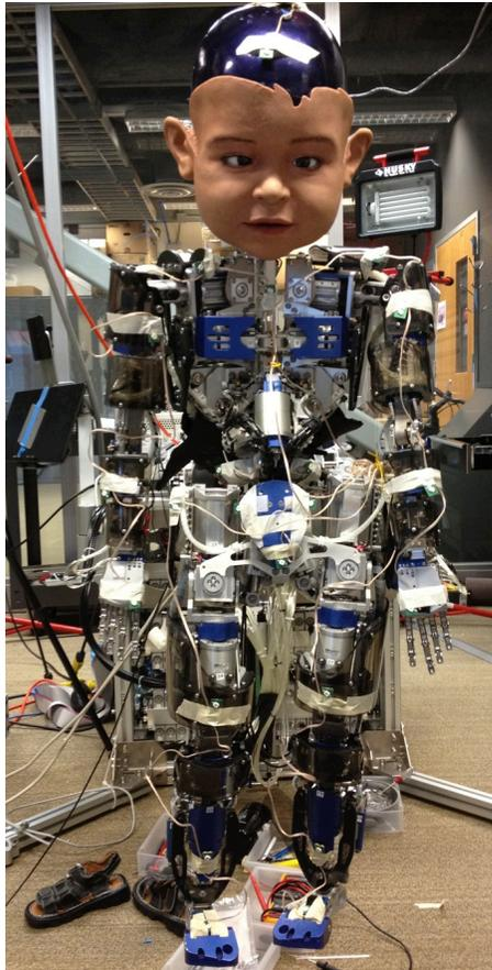
**Figure 7.1:** Diego: a humanoid robot that approximates human body complexity and dynamics.
