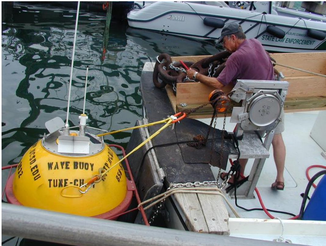
Figure 11: This gives an idea of the size of these CDIP buoys as well as the effort that goes into deploying them. A boat would tow them out to position and then drop the large clumps of chain. This scale and level of equipment is to be unused for the Dynamic Antenna System. CDIP.
