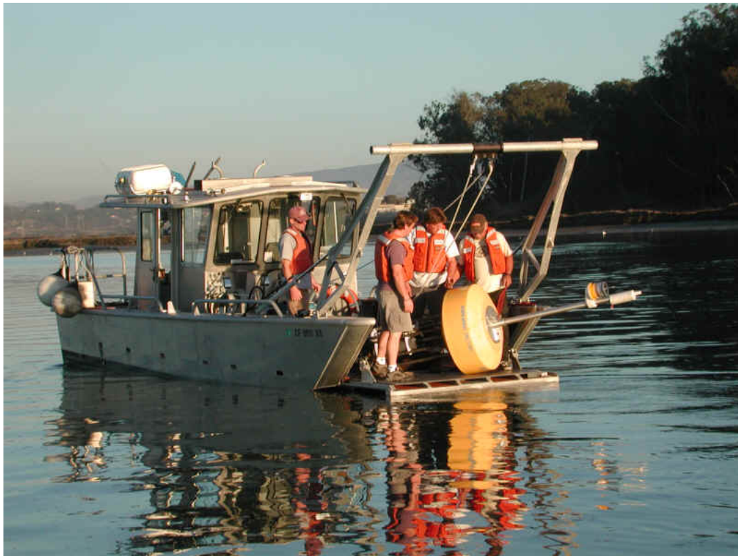
Figure 12: The deployment of a LOBO Mooring, as shown, requires a properly outfitted boat, something that the Dynamic Antenna System will be designed to not require. MBARI.
