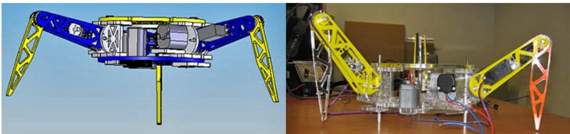
Figure 2.2: Triped robot concept pre-production on left, actual built triped robot post-production
