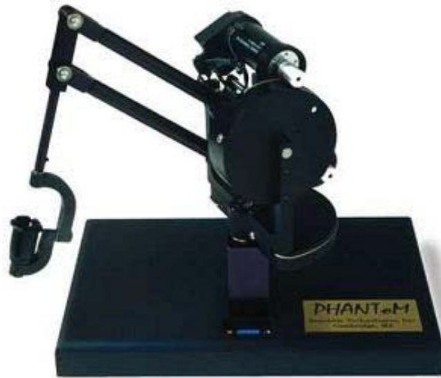
Figure 1.3: Example of a fully cable driven Phantom robot.
