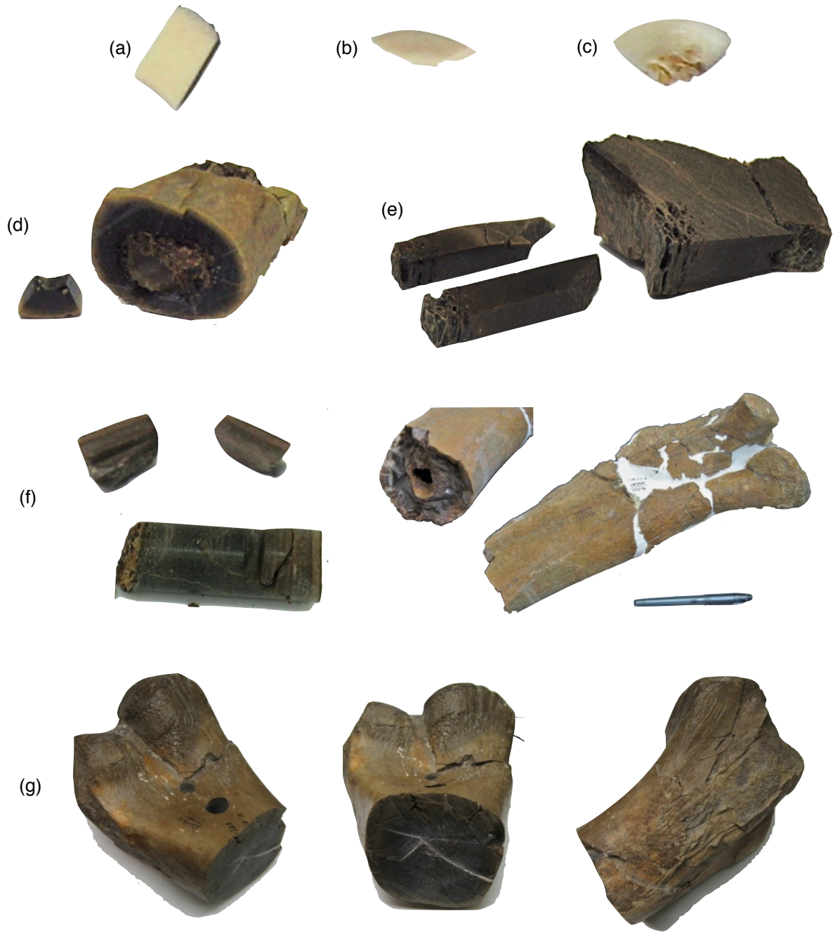
Figure 2.1 Photographs of polished bulk specimen sections, prepared for SEM, electron microprobe, and XRD. (a) Struthio (125001), (b) Rhea (UCMP 129668), (c) Caiman (UCMP 63533), (d) Pristichampsus (UCMP 170767), (e) Tyrannosaurus (UCMP 136517), (f) hadrosaur radius (UCMP 175247), (g) hadrosaur femur (UCMP 169073).
