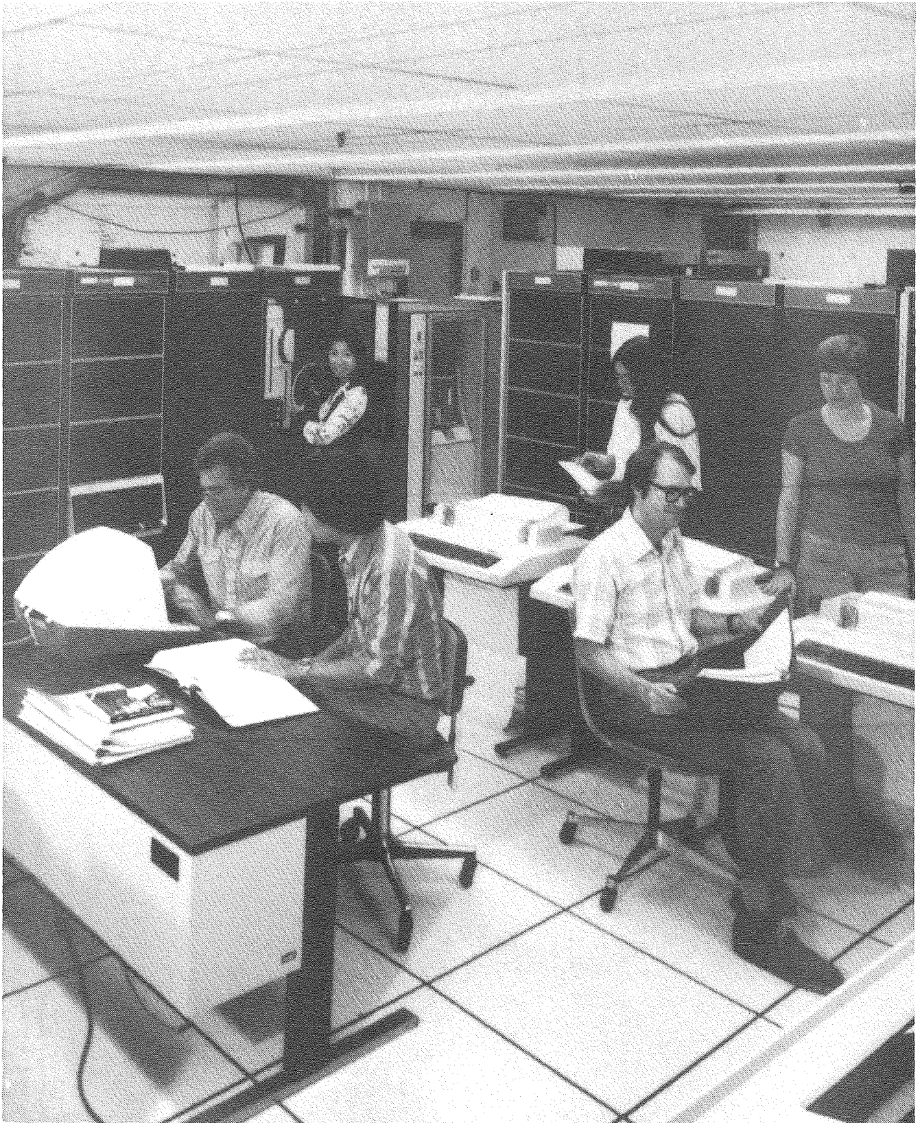
A prototyping network comprised of three minicomputers serves as a "test bed" for investigating alternatives for DOE intersite networking, and for distributed computing. Seated are (l to r) Don Austin, Carl Quong, and Bill Greiman; standing (l to r), Helena Gin, Lesta Nadel, and Rosemary Allen.
