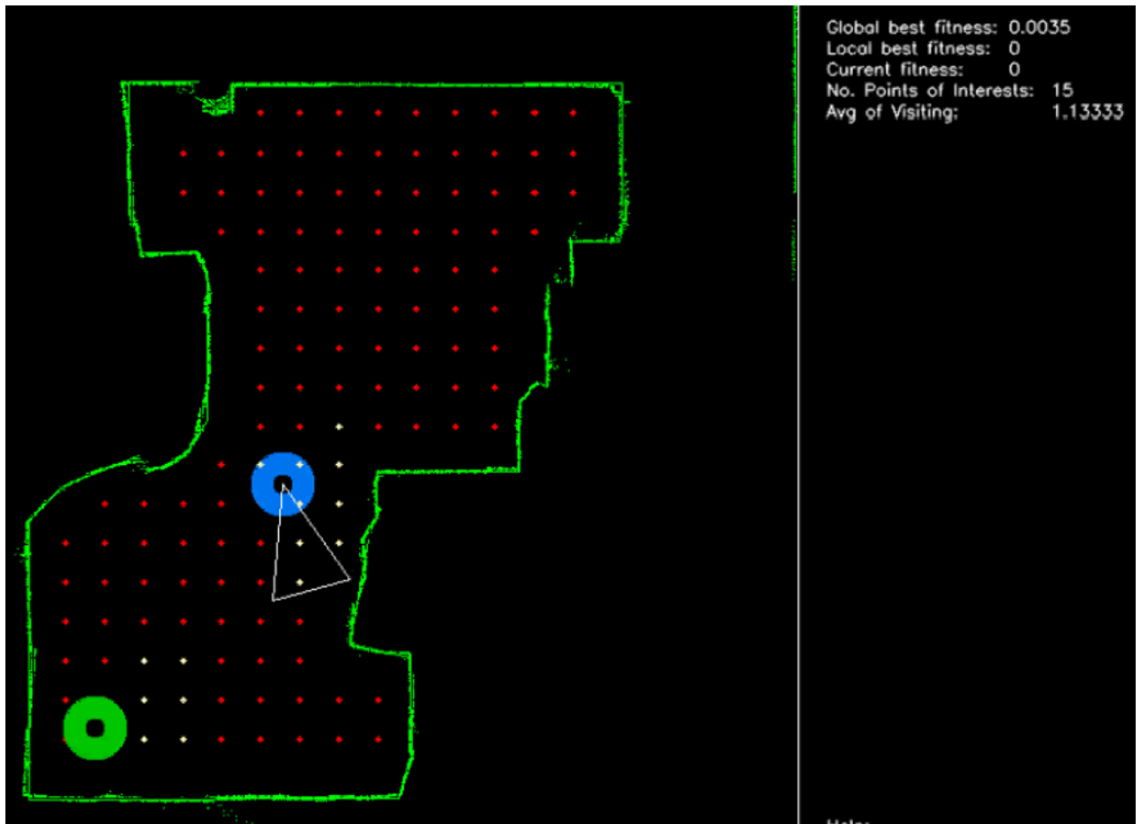
Figure 3.7. Simulator running on PeopleBot robot. Map boundaries are shown in green points and lines. PeopleBot and P3At are shown in blue and green circles respectively. Some of the PeopleBot's variables are shown on upper right section of the figure. Best global fitness variable for PeopleBot is updated by P3AT and both robots are exchanging their visited cells.
