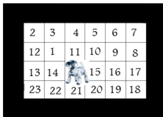
Figure 3.8. An example of exhaustive search: the numbers in the units indicate the order that the unit is going to be visited.
