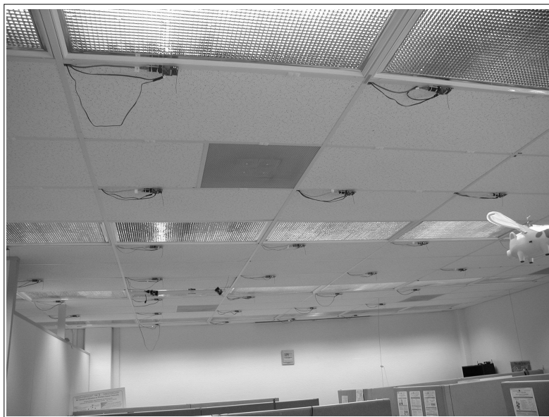
Figure 5. Fifty-five wireless network interfaces, mounted on the ceiling of our laboratory and wired back to a simulation server, help to bridge the gap between simulation and reality. Developers can learn about the effects of real wireless channels in an environment as convenient as simulation.
