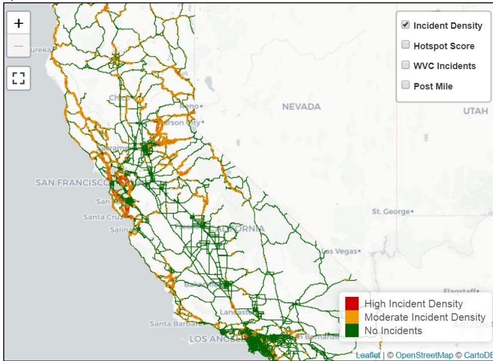
Figure 2. Automated production of a Leaflet map (.html file) showing the calculation of (a) WVC incident density and (b) WVC incident clustering for California highways.
