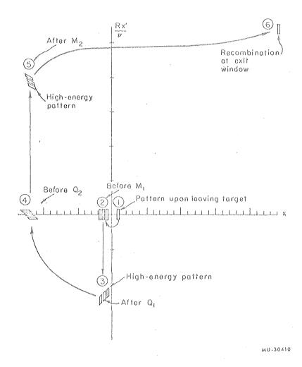
Fig. 10. Configuration pattern motion in radial phase space.
