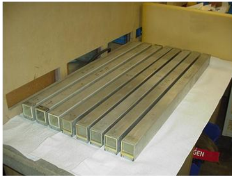
Figure 15 NaI(Tl) scintillator bars
