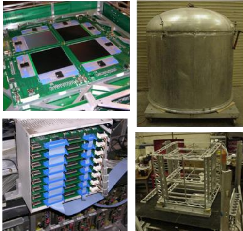
Figure 11(cw) Single Si layer, pressure vessel, detector support structure and bias control box.
