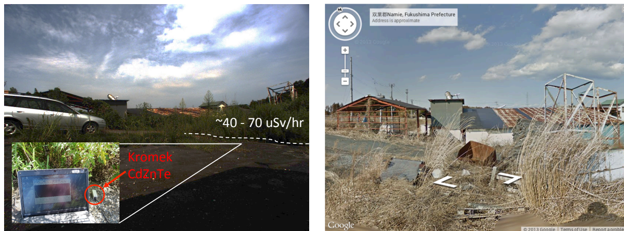
Figure 6.8: Image near the Site 1 staging area taken with the HEMI auxiliary camera, left. Areas of high activity were detected with handheld meters, as indicated by the dashed white lines. The image on the right was taken of the same area using Google Street View Car around March of 2013 (image courtesy Google).
