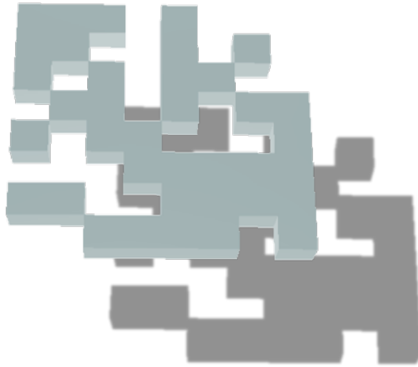
Figure 2.5: Illustration of the coded-aperture technique. A far-field source of radioactive emission casts a shadow of the mask pattern onto a focal plane. The resulting pattern can be used to identify the location of the source.
