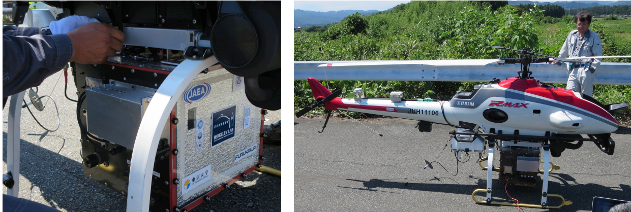
Figure 6.5: The HEMI instrument enclosure during mounting to the UAV, left, and the Yamaha RMax with the HEMI payload prior to take-off for the first flight measurement, right.
