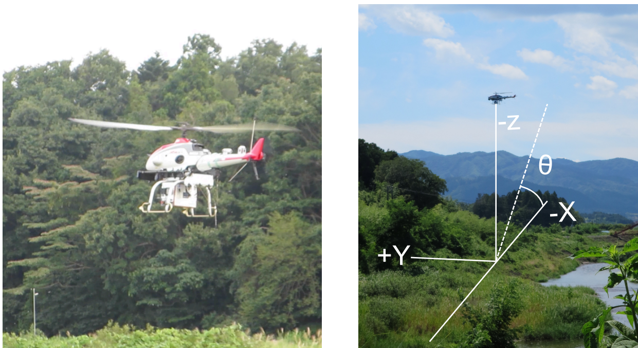
Figure 6.6: The HEMI instrument in flight. Coordinate system with respect to ground during hover measurements at Site 1 is shown, right.
