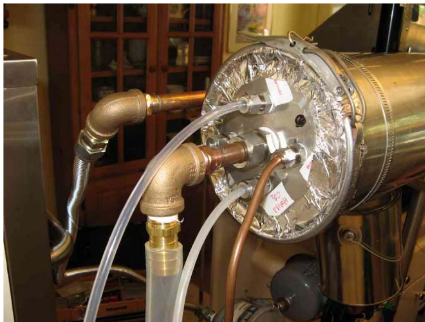
Figure 4. Outlet of dilution sampling system
