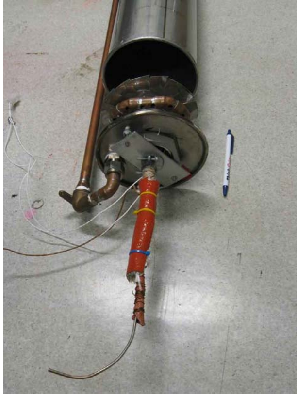
Figure 3. Dilution sampler inlet configuration
