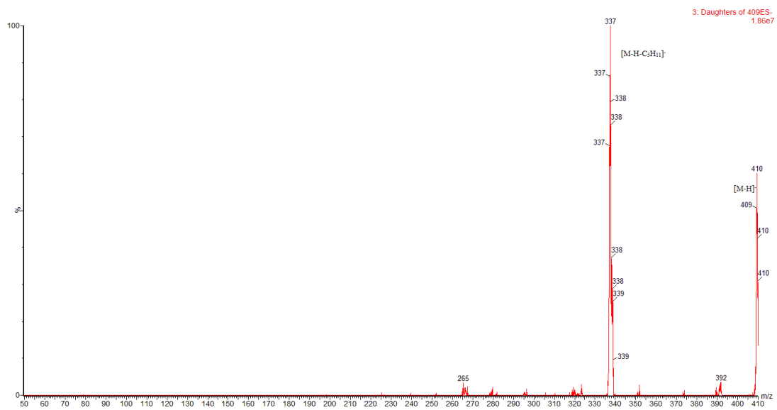
Figure S 5-44 UPLC-MS-MS spectra of OP-3-2B at retention time 9.79 min, dimer of octylphenol
