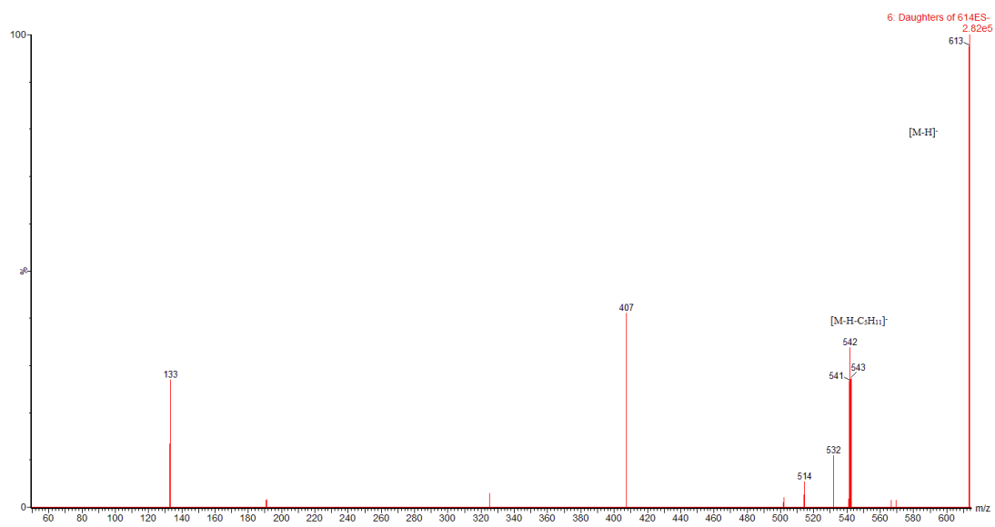
Figure S 5-42 UPLC-MS-MS spectra of OP-3-1C at retention time 10.65 min, trimmer of octylphenol
