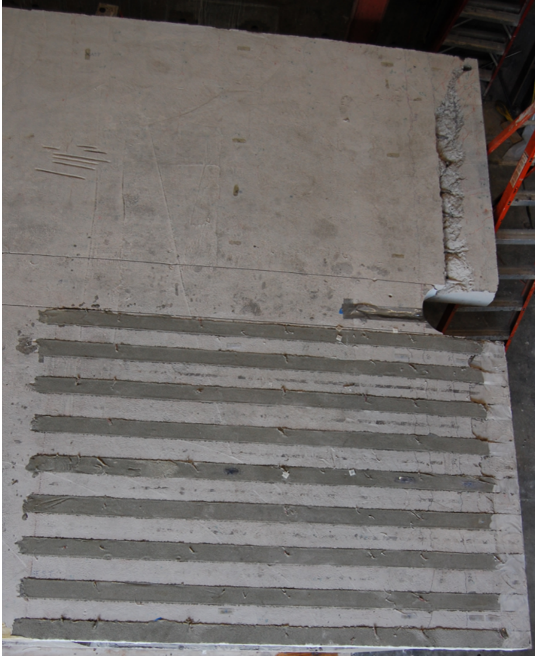
Figure 6.67 Top view of deck slab tested to ultimate capacity after removal of loose concrete
