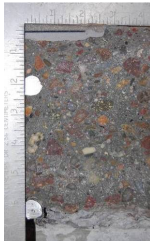
Figure 6.57 Detail showing actual location of reinforcement
