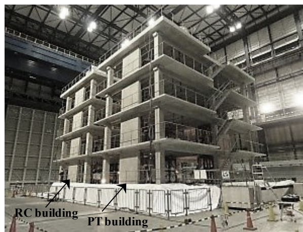
Figure 4-3 RC and PT buildings on shake table
