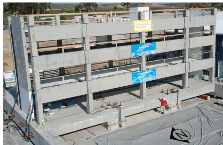
Figure 2-10 Half-scale, three-story, precast building on shake table at University of California, San Diego
