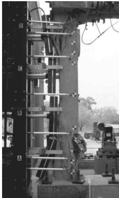
Figure 3.48: Progressing Shear Cracks (Test 7, 41.7 ms)
