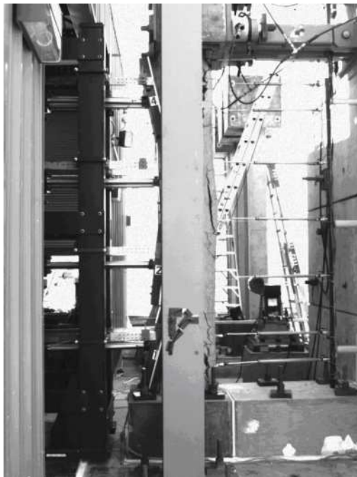
Figure 3.9: Rear Face Spalling (Test 2, 15.4 ms )
