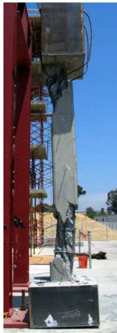
Figure 3.63: Specimen Post-Test (Test 8, removed from test fixture)
