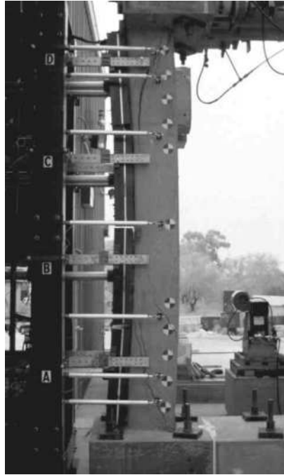
Figure 3.47: Progressing Shear Cracks (Test 7, 6.7 ms)
