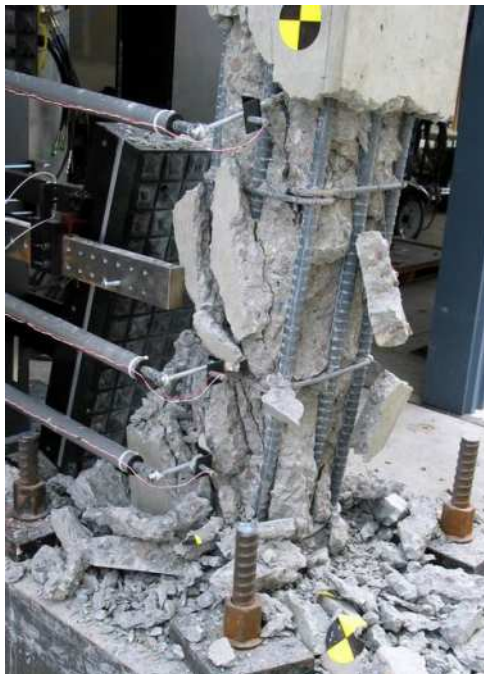
Figure 3.54: Bottom Damage Detail (Test 7)
