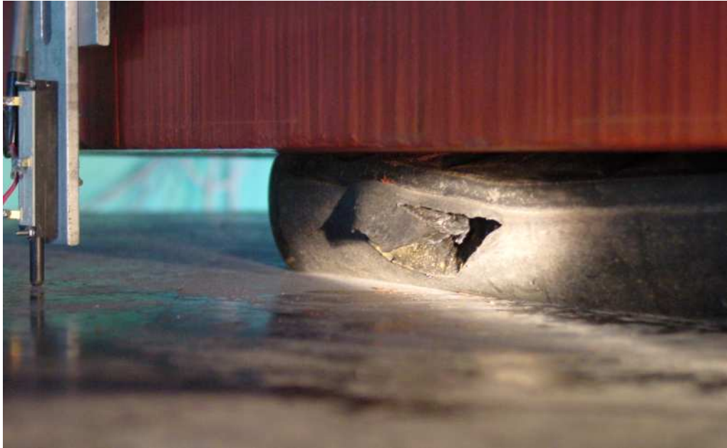
Figure 4.9: Local Damage Observed in Programmer Tests
