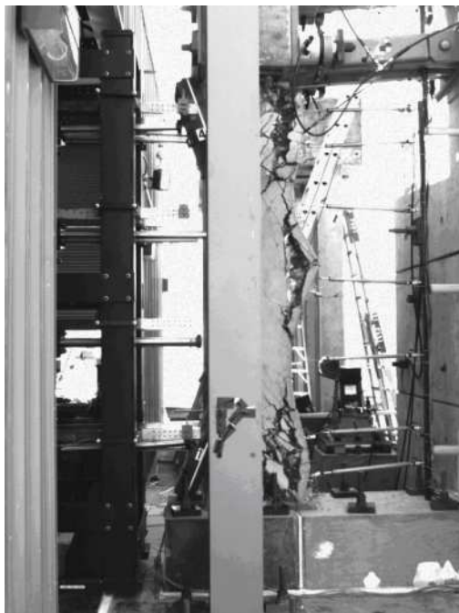
Figure 3.10: Column Failure (Test 2, 35.4 ms)
